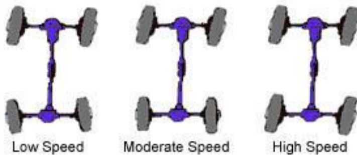
Figure 2: Speed dependent rear wheel steering. (Image Source: General, n.d.).
