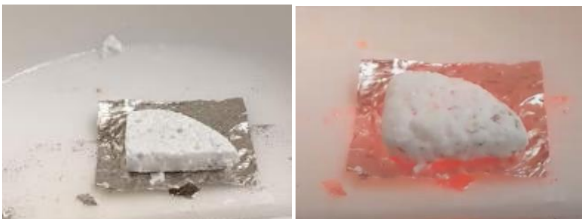
Figure 4.11: Pressed, polished, and sectioned YbBO 3 puck piece (Left) swelling after 10 min exposure at 1200°C in stagnant air box furnace (Right).
