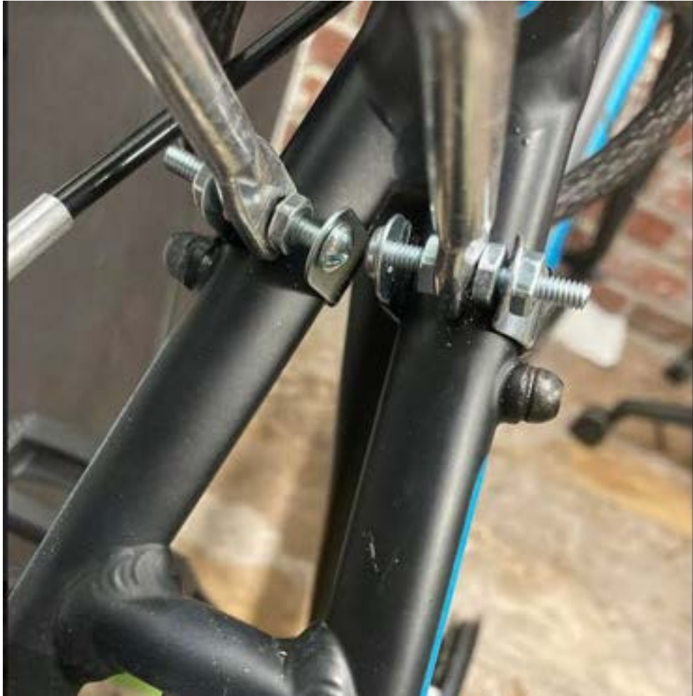
Figure 27. Securing of Bike Rack
