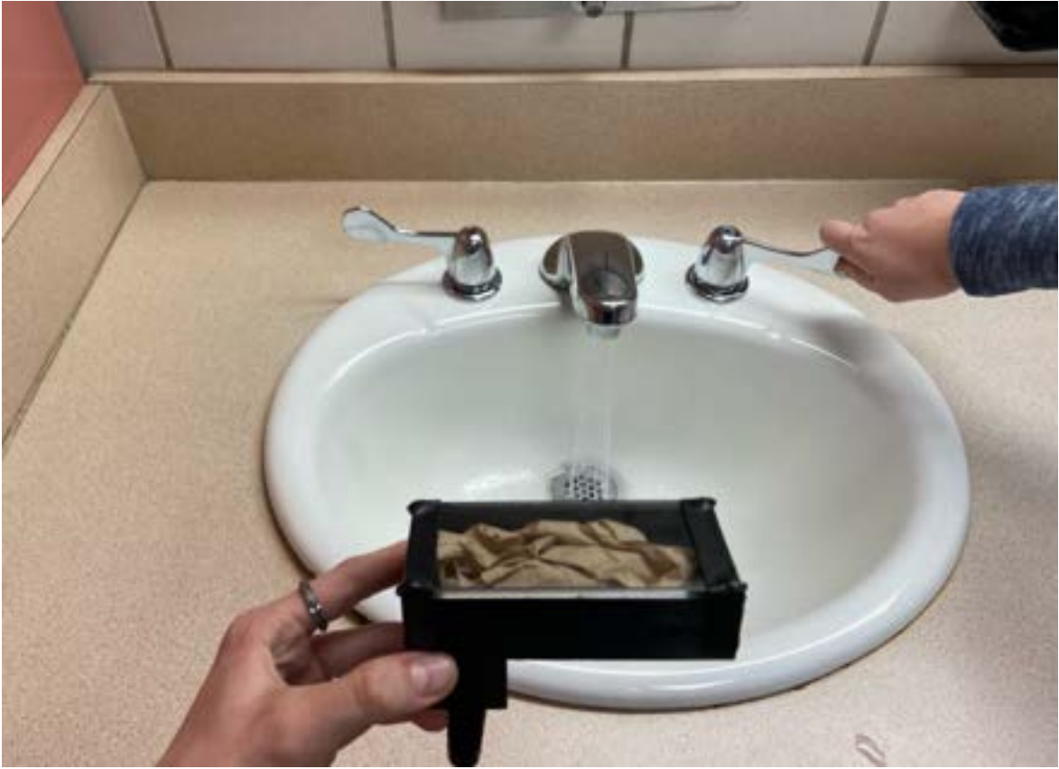
Figure 39. Front Box Waterproof Testing with Napkin
