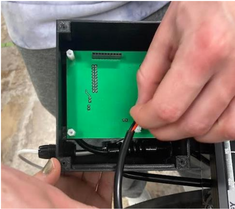
Figure 26. Construction of Back Box
