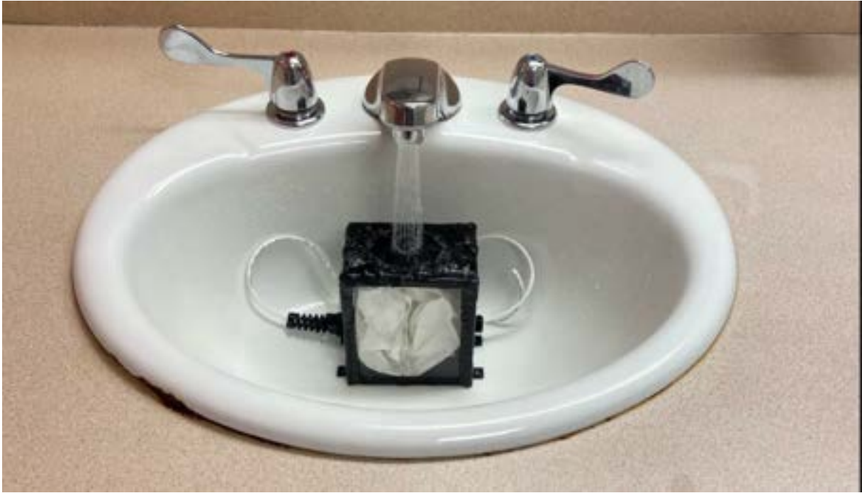
Figure 38. Back Box Waterproof Testing with Napkin
