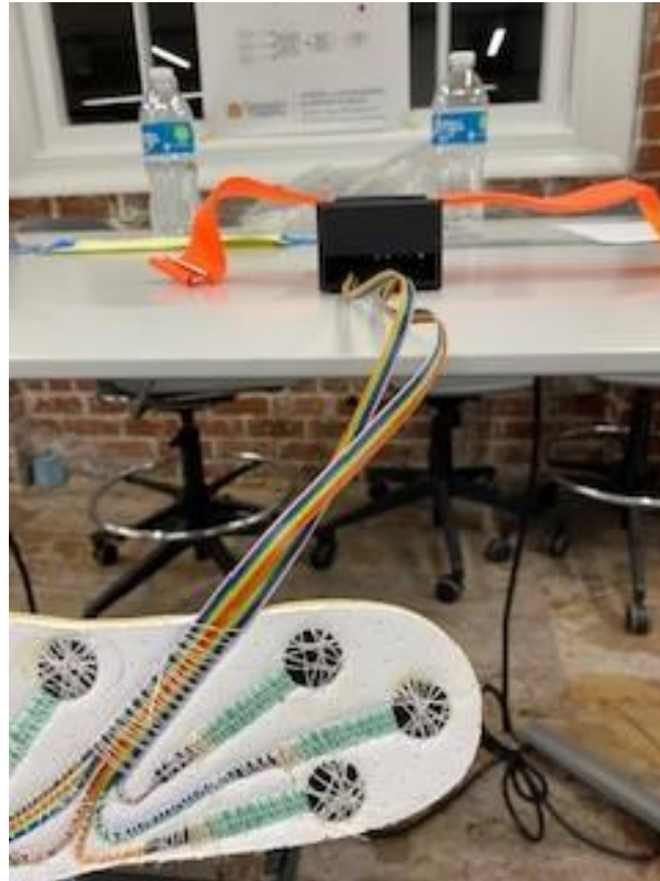
Figure 35: Shoe Sole Sensor Placement
