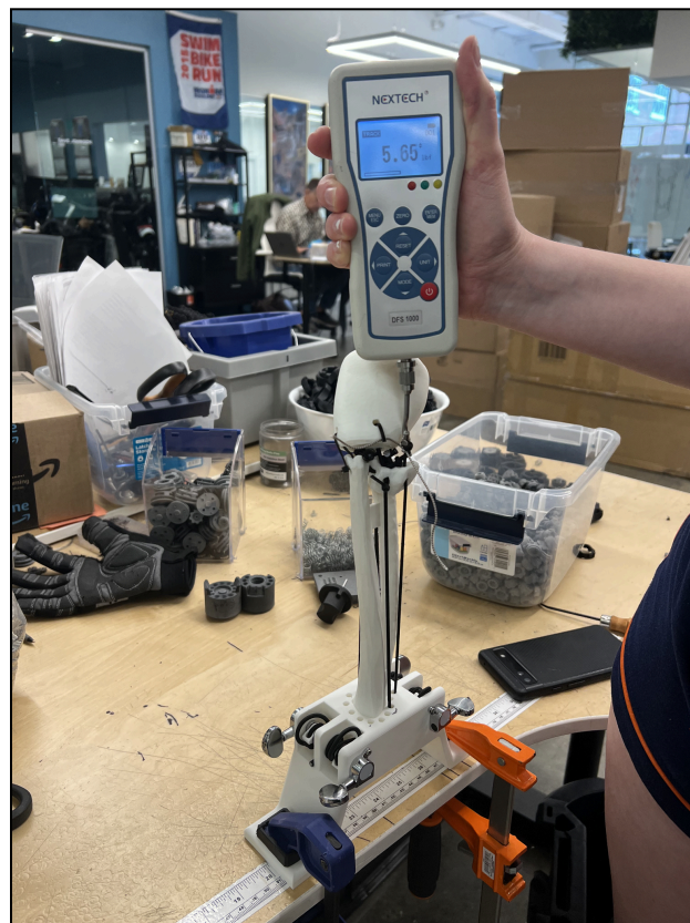
Figure 20 Setup for tensile testing of the 4 different elastics
