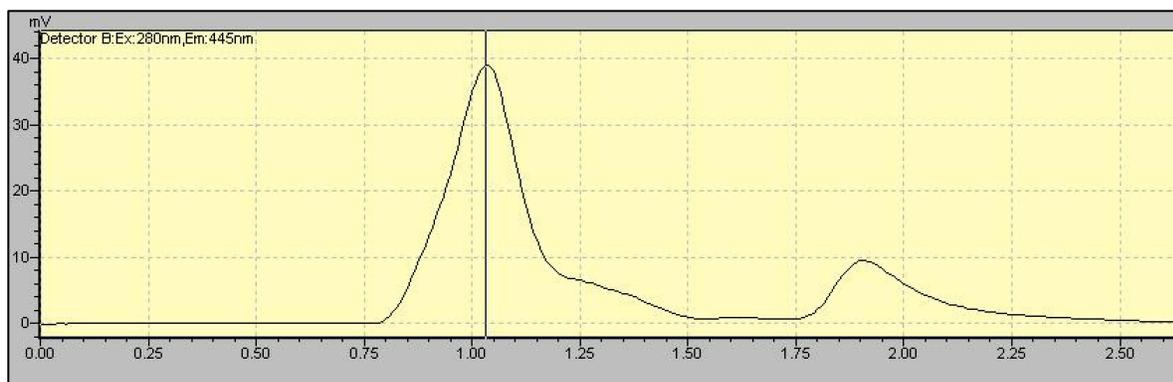
**Figure 4-3.** Example chromatogram for 80  $\mu$ g/L CIP standard in a mixed solution of formic acid/acetonitrile/methanol (2/49/49) under HPLC (Shimadzu) fluorescence detection. CIP elutes at roughly 1.9 minutes. Formic acid in the mobile phase generates a peak at roughly 1.0 minute.
