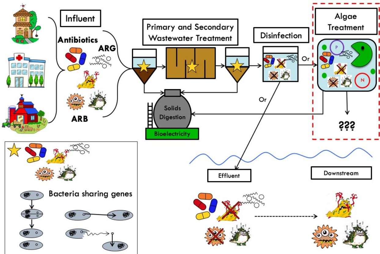
**Figure 1-2.** The pathway for antibiotic resistance-stimulating constituents to enter the wastewater treatment system and disseminate through effluents into the environment. This dissertation seeks to evaluate the potential role of an algae treatment system in mitigating antibiotics and ARGs. The star symbol represents areas of the wastewater treatment system where ARB are selectively amplified through both vertical and horizontal gene transfer processes.
