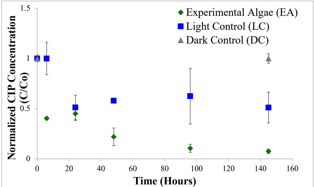
**Figure 3-1.** Normalized ( $C/C_0$ ) concentrations of ciprofloxacin (CIP) over time for experimental algae (EA) and light control (LC) reactors over 144 hours. For dark control (DC) reactors, CIP concentration measurements were taken at hours 0 and 144. Normalized CIP concentrations refer to CIP concentrations at time =  $t$  divided by initial CIP concentration ( $C_0$ ), where  $C_0 = 25 \mu\text{g/L}$ . Error bars are standard error for triplicate reactors of each condition.
