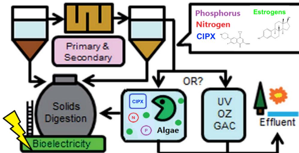
**Figure 1-1.** Diagram of an integrated algae-WWTP system including both nutrient and unregulated contaminant removals and energy generation from methane-derived electricity (Zhang et al., 2014).
