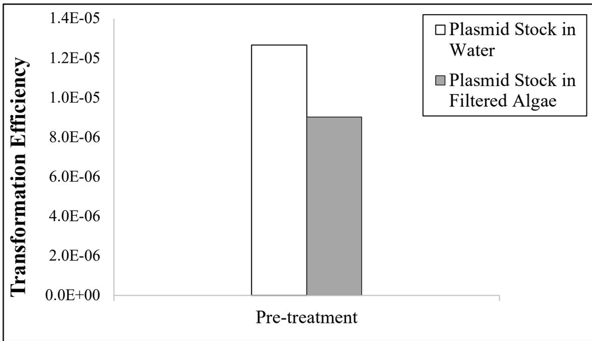
**Figure 5-3.** Preliminary transformation efficiencies of 3.48 ng/ $\mu$ L pEX18Tc plasmid standards in nuclease-free water and filtered algae background matrix. See Equation 5-1 for the transformation efficiency equation.
