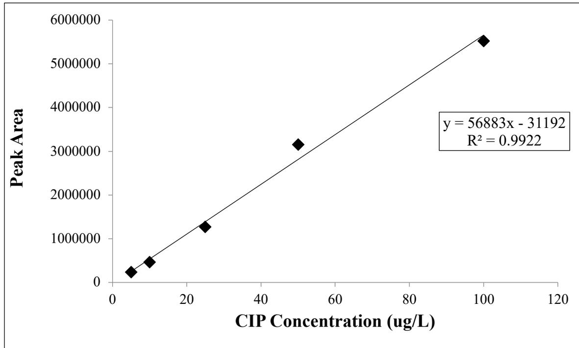
**Figure 4-4.** Calibration curve for CIP concentrations over the range 2-100  $\mu\text{g/L}$ . The minimum detection level of CIP for this method was 2  $\mu\text{g/L}$ .
