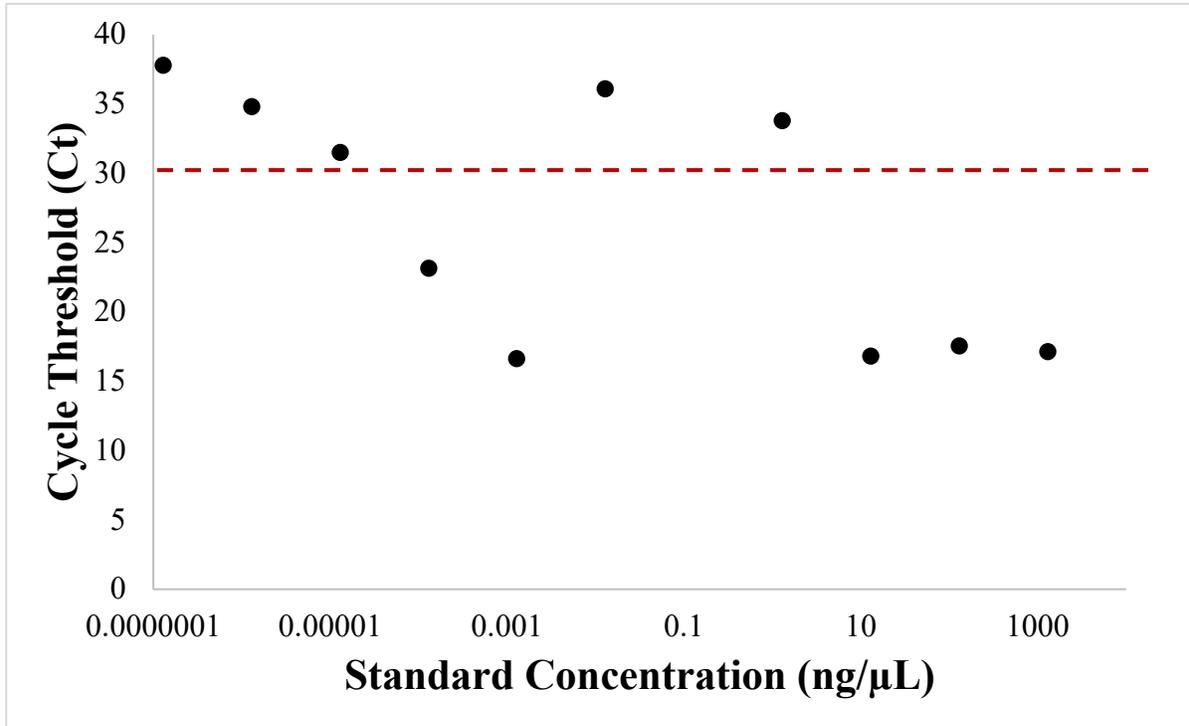
**Figure 5-2.** Preliminary qPCR standard curve using short amplicon primers for plasmid pEX18Tc. There was no calibratable region for this qPCR run and the red dashed line denotes the qPCR detection limit (Ct = 30 cycles). Standard concentrations are presented in Table 5-3.
