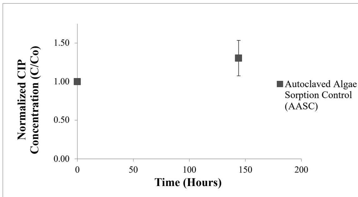
**Figure 4-2.** Normalized ( $C/C_0$ ) concentrations of ciprofloxacin (CIP) over time for autoclaved algae sorption control (AASC) reactors over 144 hours. Error bars are standard error for the duplicate AASC reactors.
