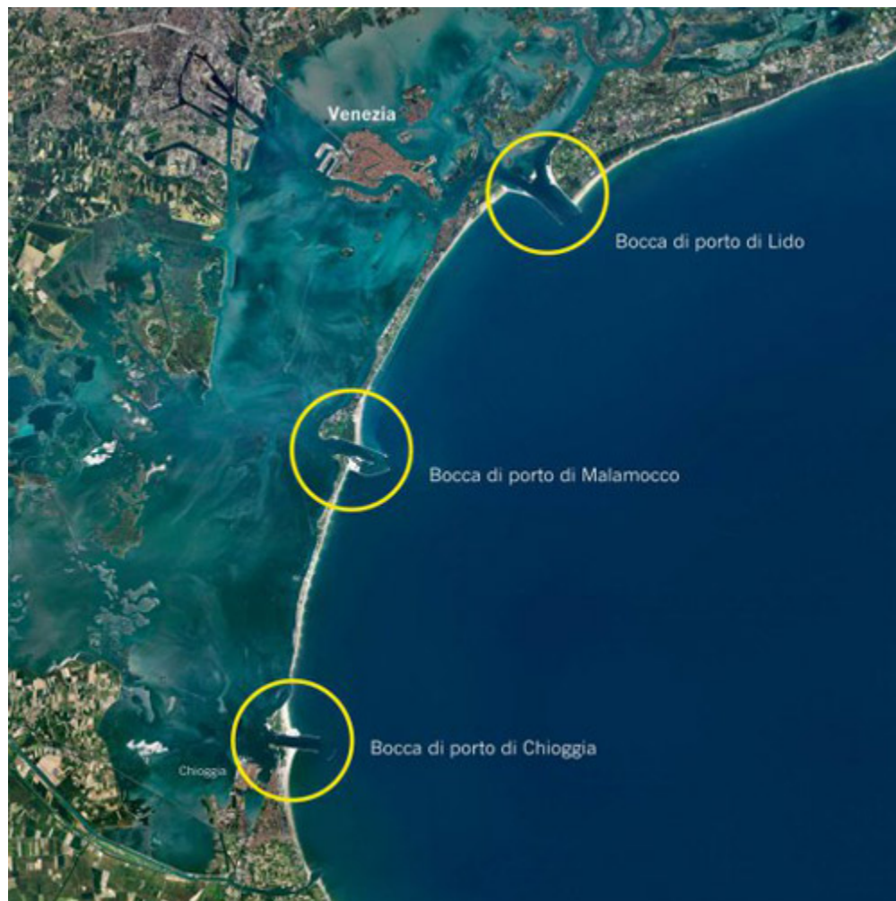
Figure 2: The Modulo Sperimentale Elettromeccanico (MOSE) system is a series of retractable barriers which cover the inlets of Lido, Malamocco and Chioggia (“MOSE System”, n.d.).
