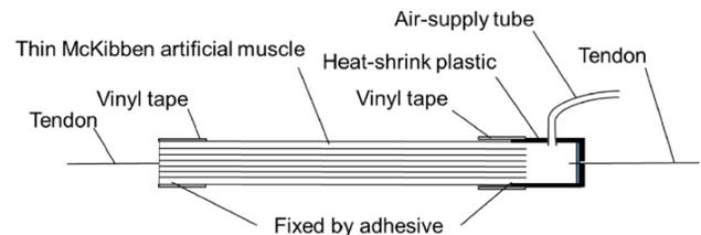
Fig. 10. Multifilament connection diagram [4].
