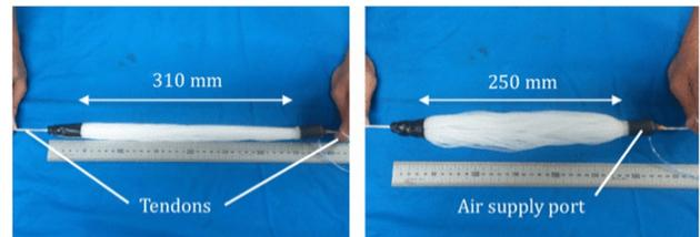
Fig. 9. Contraction of multifilament muscle [4].
