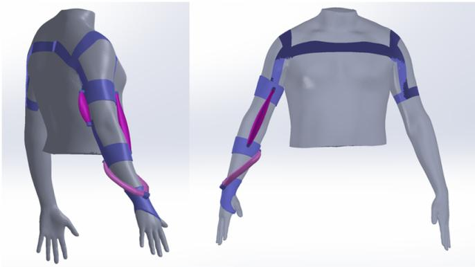
Fig. 11. 3D Visualization of elbow joint actuators and framework.
