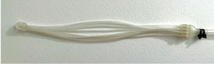
Fig. 16. Final design of the multifilament Thin McKibben muscle.
