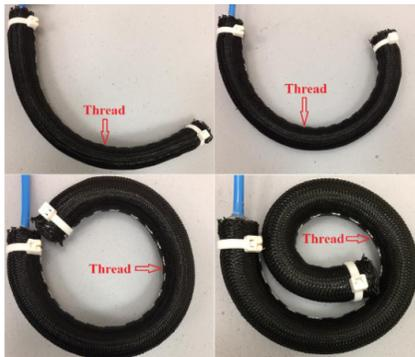
Fig. 5. Image of Extensor-Bending Pneumatic Artificial Muscle (EBPAM) [2].
