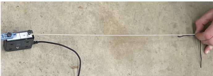
Fig. 14. Singular Thin McKibben muscle attached to a force tester.
