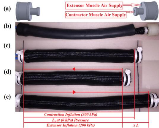
Fig. 3. Parts of novel Extensor-Contractor Pneumatic Artificial Muscle (ECPAM) [2].
