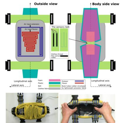
Fig. 7. Image and diagram of Soft Exosuit for Elbow Assistance [3].
