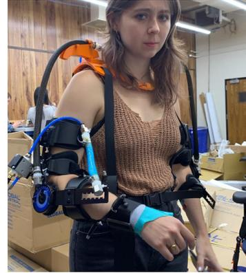
Fig. 20. Combined elbow exoskeleton and shoulder exoskeleton setup.
