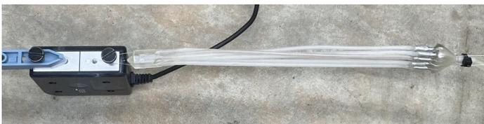
Fig. 22. Force testing setup for multifilament muscles.
