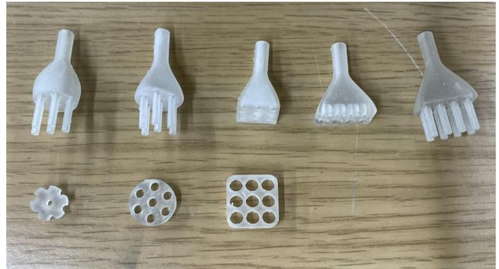
Fig. 15. Several iterations of the multifilament Thin McKibben connector.
