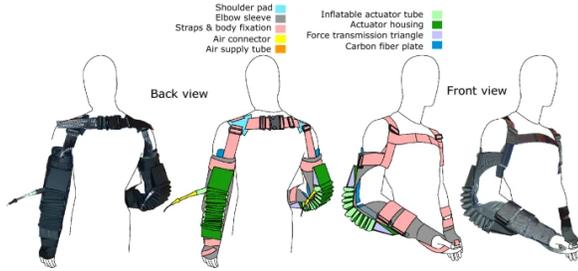
Fig. 1. Carry exoskeleton diagram [1].
