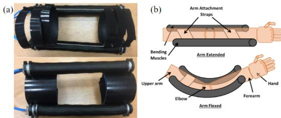
Fig. 6. Image and diagram of Elbow Rehabilitation Exoskeleton [2].
