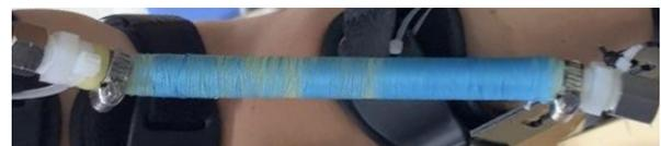
Fig. 19. Inverse Pneumatic Artificial Muscle.
