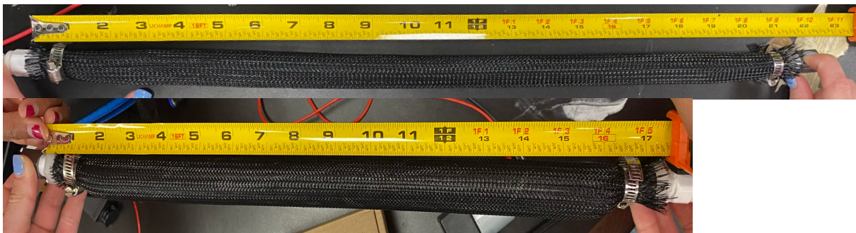
Fig. 18. Muscle one contraction testing. 21” resting (top) and 16.75” at maximum contraction (bottom).
