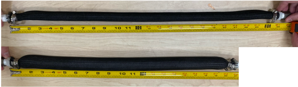
Fig. 19. Muscle two contraction testing. 24.5” resting (top) and 20” after contraction (bottom).
