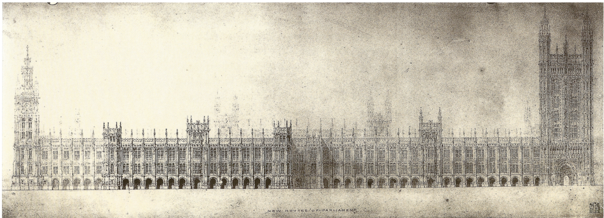
Figure 13: Barry's elevation of the west front. Note regularity and organization of façade. Turrets create even bays.
