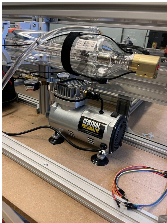
Figure 11: Head of the Laser Tube and Air Compressor
