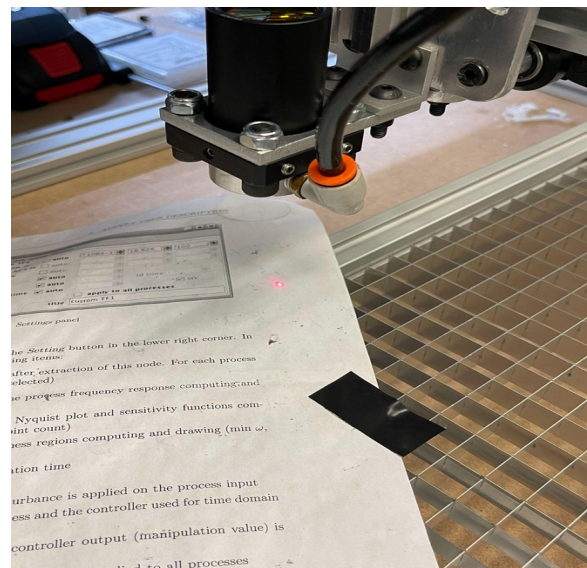
Figure 13: Laser Beam Exiting Laser Head Assembly
