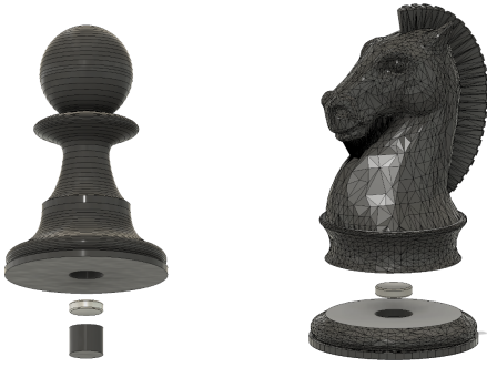
Fig. 13. Initial chess piece design with a slot and plug (left) and final design with a base and body (right).
