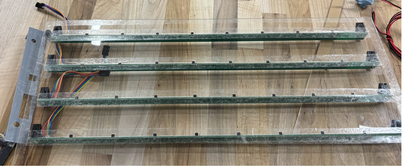
Fig. 5. Sensor boards installed into the acrylic surface sheet.
