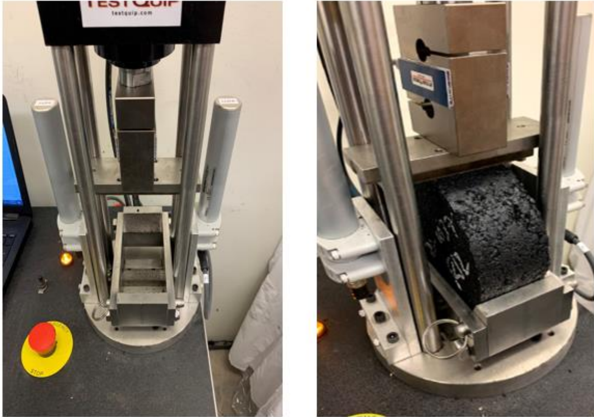
Figure 5 - IDEAL-RT setup with u-shape fixture
