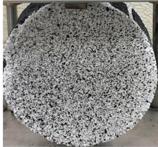
Speckle pattern using spray paint technique
