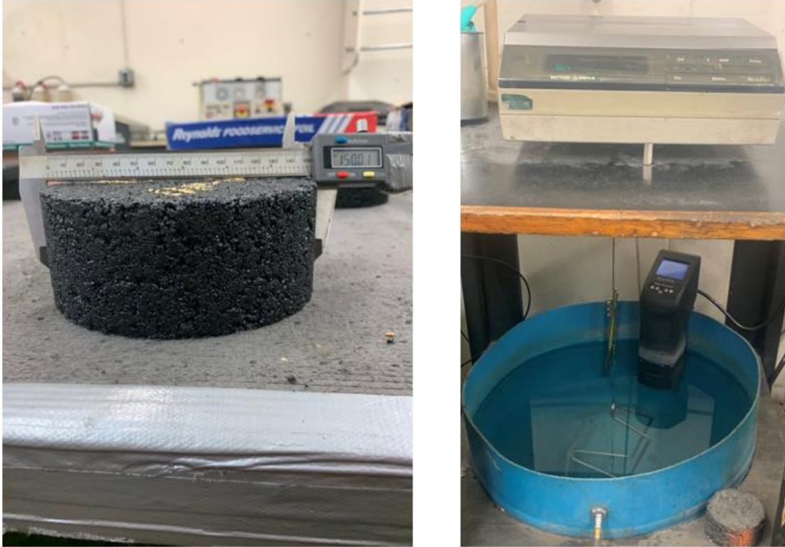
Figure 8 - Specimen measurements and air voids determined as part of specimen preparation process
