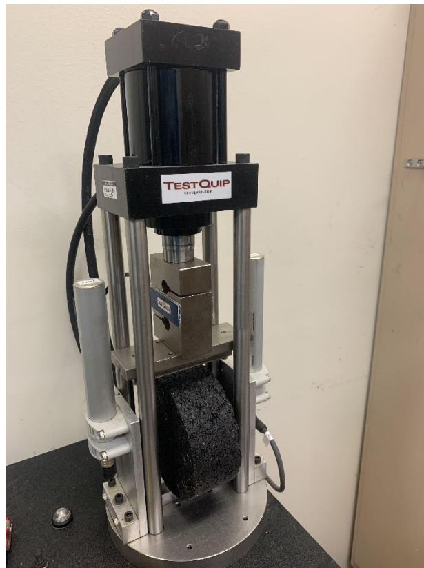
Figure 1 - IDT test setup for rutting evaluation
