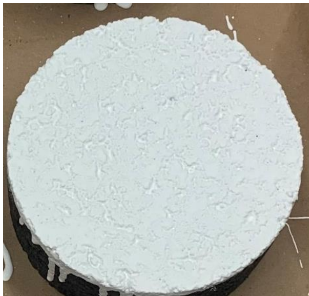
Figure 53 - White surface of DIC specimen
