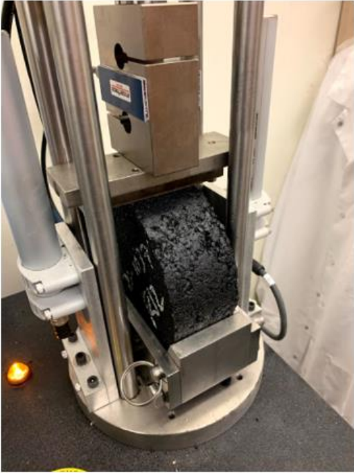
Figure 11 - IDEAL-RT setup and example of resulting load vs. displacement curve
