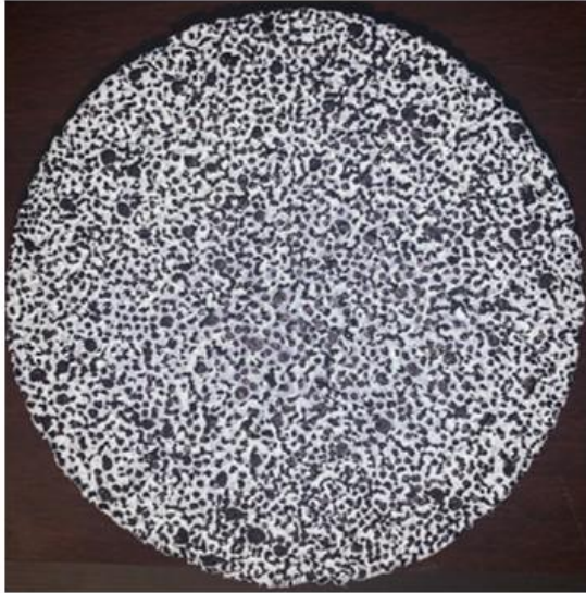
Speckle pattern by hand with permanent marker
