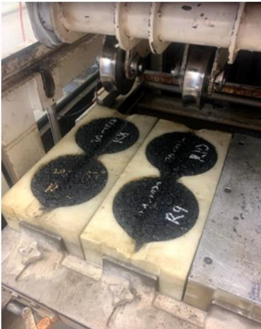
Figure 9 - APA test setup and example of results
