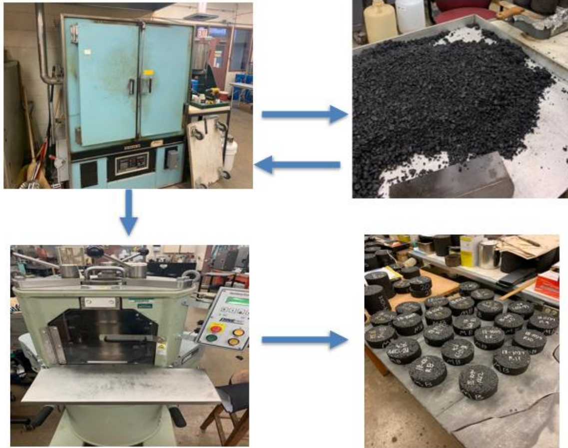
Figure 7 - Asphalt specimen preparation for Phase 1
