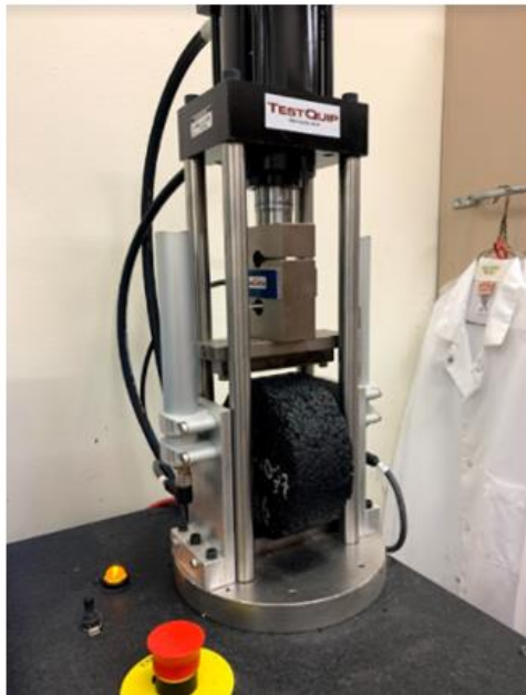
Figure 10 - IDT test setup and example of resulting load vs. displacement curve
