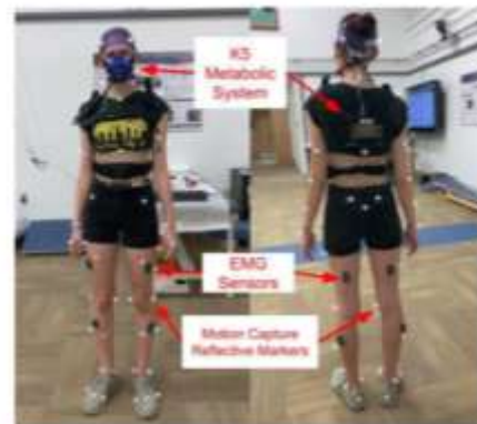
Figure 5. Standard Equipment for MAMP Lab Motion Capture Studies. Images showing motion capture equipment worn by each subject during data collection. Design of the pulley system and accompanying belt needed to be compatible with existing equipment.
