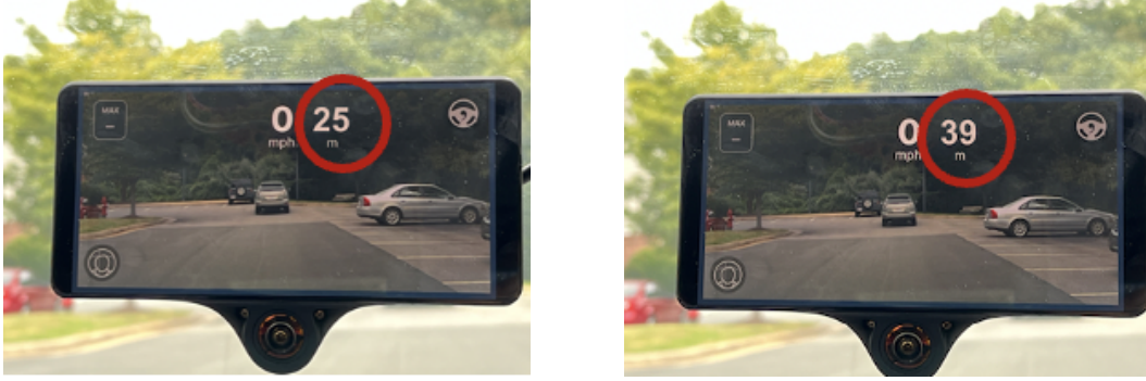
Figure 4.19: Evaluation on an actual car in a parking lot: relative distance predictions (Left) without and (Right) with adding an adversarial patch.
