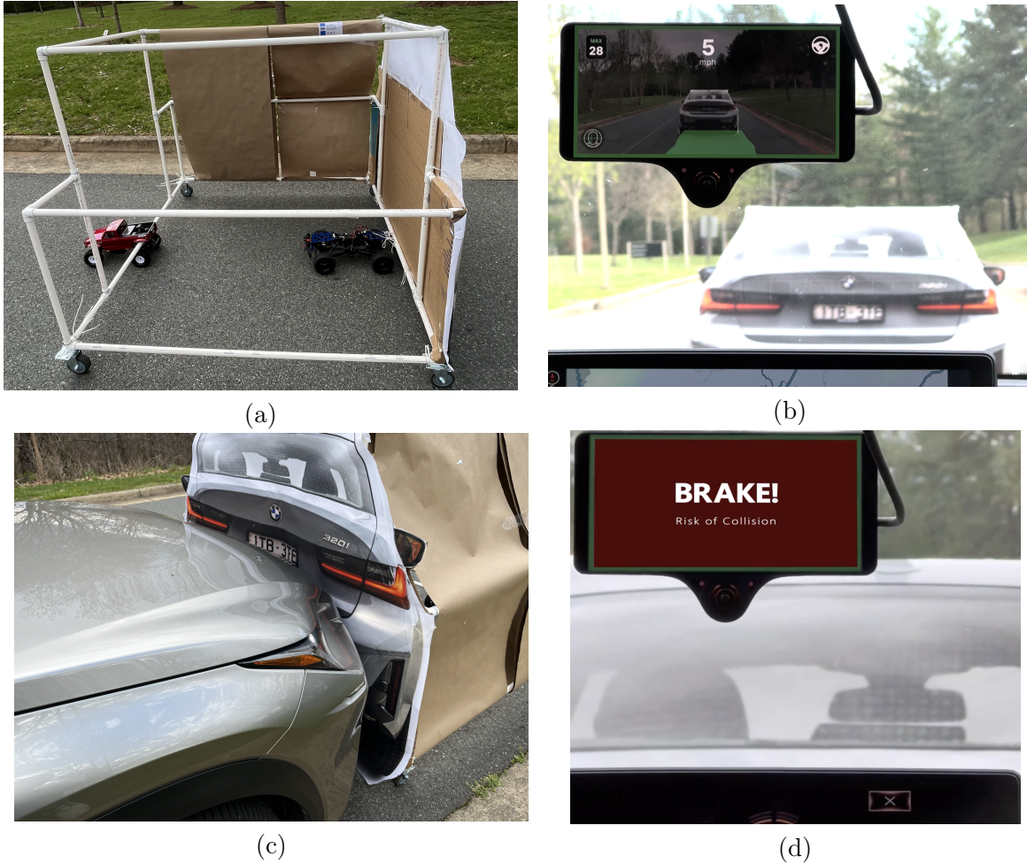
Figure 4.21: (a) Side view of lead car model; (b) AV follows the car model in a benign scenario; (c) AV under perception attack collides with the lead car model; (d) Driver's view upon collision.
