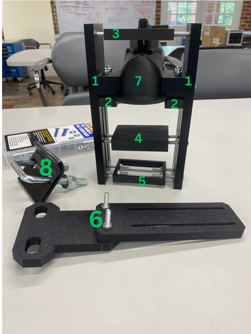
Figure 13: Sensor Mount Assembly
