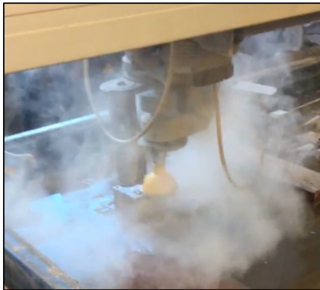
Figure 5. Waterjet Blasting into an Aluminum Block.
