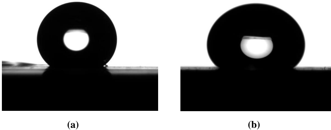
Fig. 54: Water drop sitting on PDMS covered one scan surface of (a) glass and (b) aluminum.
