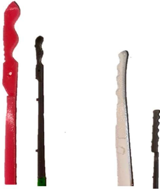
Fig. 6. Scale Comparison of Blades. The two final iterations with the larger, scaled-up 3D printed version on the left and the to-scale SLA resin printed blade on the right.
