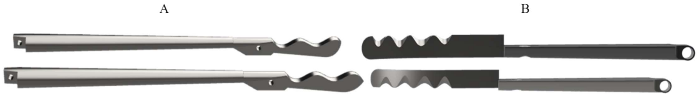
Fig. 5. Two Final Sinusoidal Design Iterations. The two final sinusoidal blades are shown in this image as CAD renderings. These final two blades were printed out of resin using SLA printing. They were used in the dry testing with the cooked pasta.
