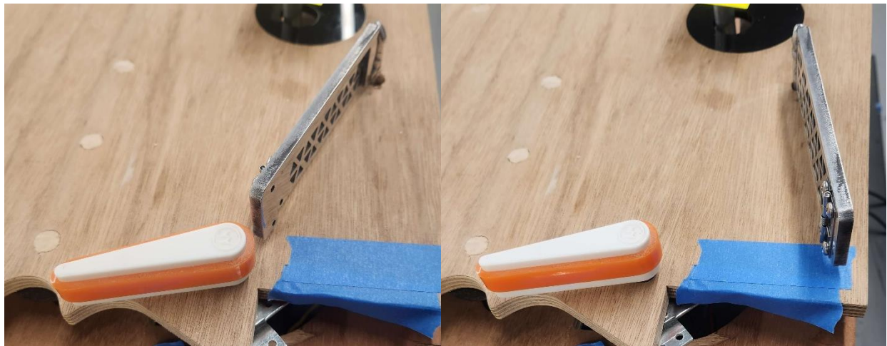
Fig. 2.5.2. Diverter gate in closed and open position
