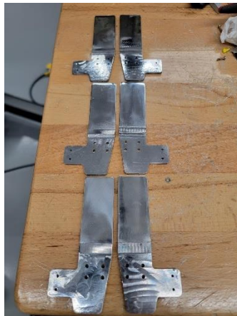
Fig. 2.2.6. Final version of polished and CNC'd aluminum drop targets
