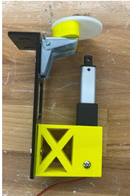
Fig. 2.6.3. First prototype of the vertical trapdoor design
