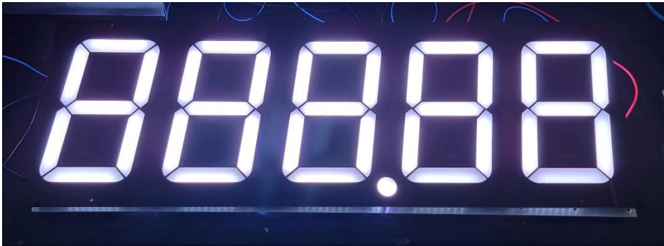
Fig. 2.10.7. Complete LED Backlit Acrylic
