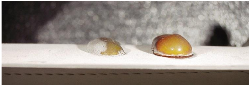
Figure 2-6. Representative image of a cured maskant on a flat, platinum-plated airfoil region.
