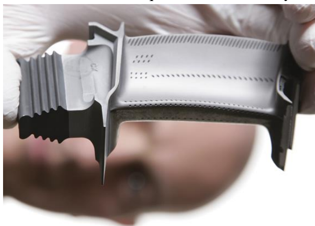
Figure 2-1. An example of a turbine blade. The ridged area on the left is the root. The curved area to the right of the airfoil is the shroud. From The Engineer Ref 15 .
