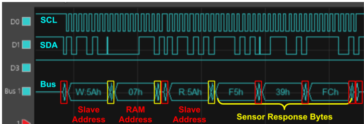
Figure 8. Screen capture of I2C communication with temperature sensor.
