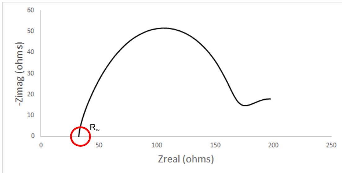
Fig. A2.4. Example of EIS results form a Li/Li symmetric cell as shown in Fig. A2.3 and R_\infty
