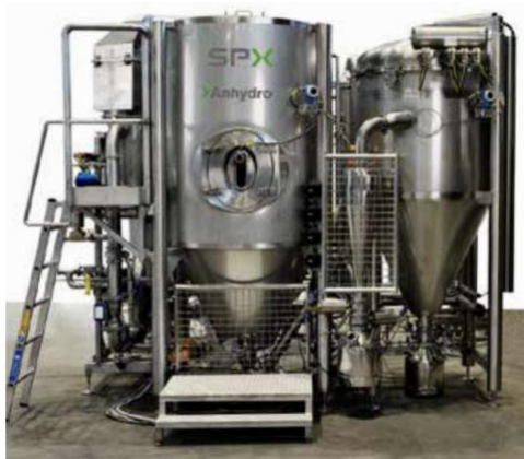
Figure 7.4.2. Pilot Scale SPX Anhydro Spray Dryer
