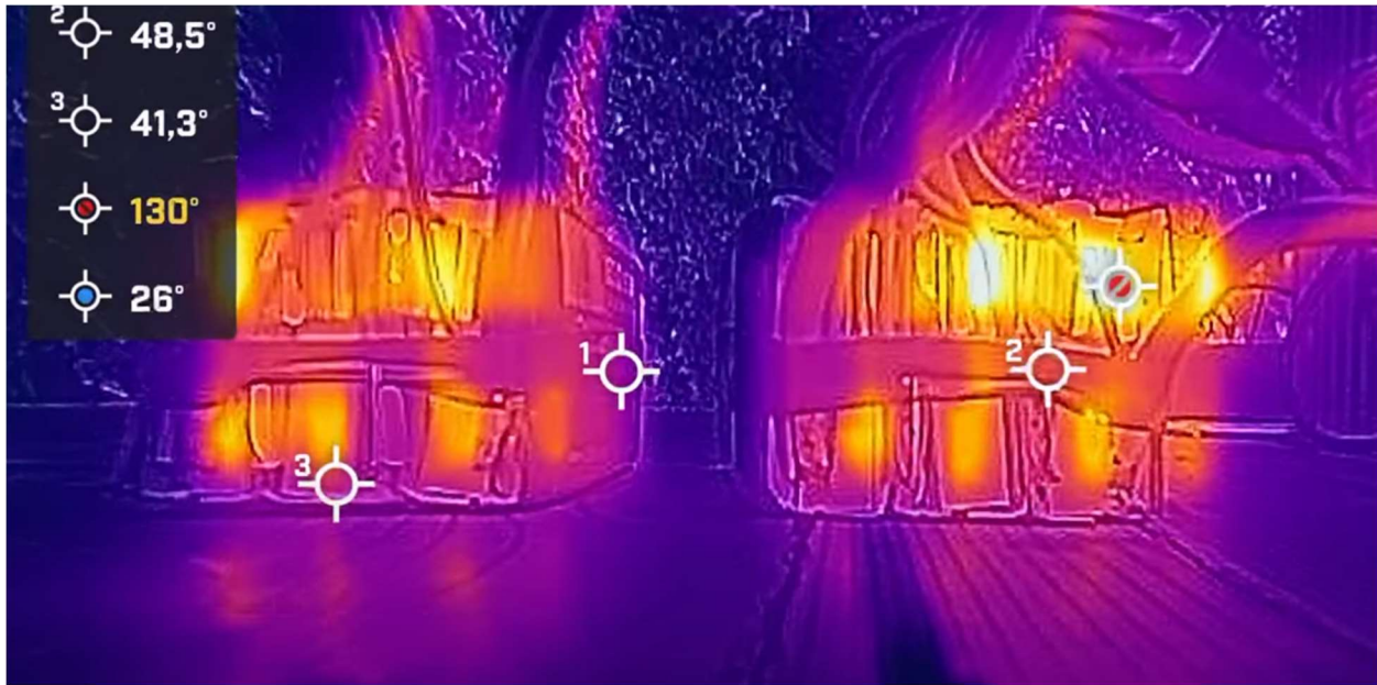
Figure 8: Thermal Imaging of LiPo Batteries under extreme loading (Bell, 2024)
