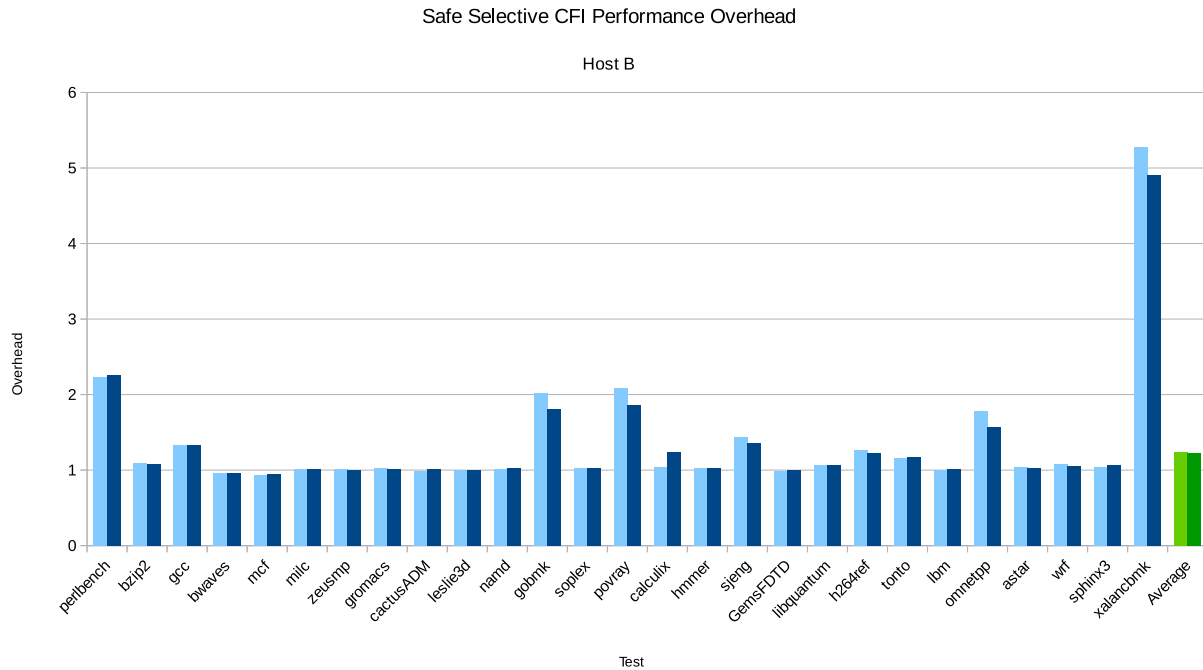
Figure 12.14: Performance overhead of the applications in the SPEC2006 benchmark suite when protected using SelectiveCFI without checking the safety of ret targets in functions statically deemed safe. These results are for Host B. The results for the applications protected with Safe SelectiveCFI are shown on the right, in dark blue and dark green. The results for the applications protected with Basic SelectiveCFI are shown on the left, in light blue and light green.
