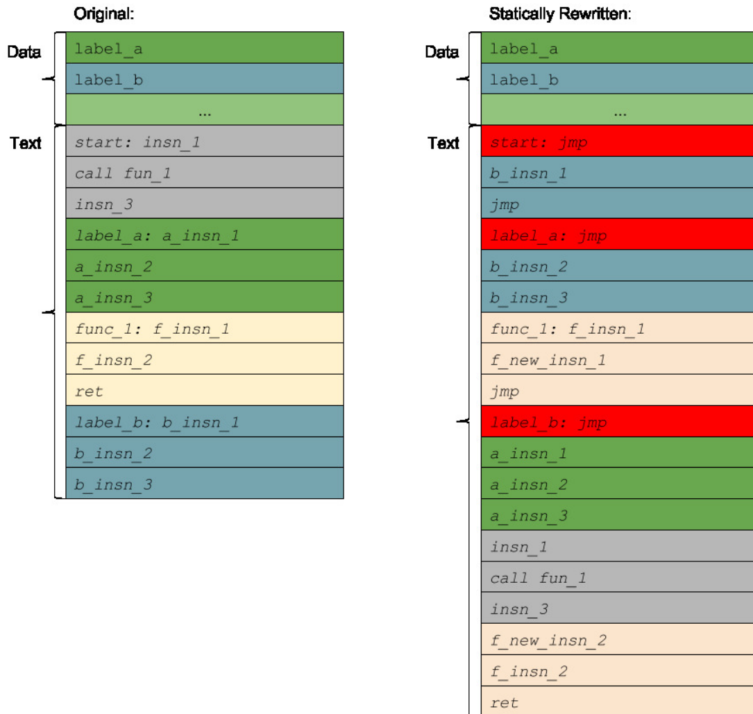
Figure 4.6: The algorithms of the Reassembly phase are one cause of overhead in the statically rewritten program/library. Shown here is the overhead of the algorithms of the Reassembly phase from links at pinned addresses and dollop splitting and the overhead from User-specified transformations.
