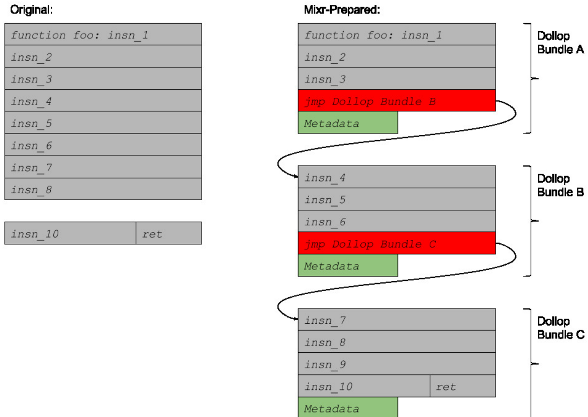
Figure 10.3: Creation of dollop bundles from straight line code in the original program.
