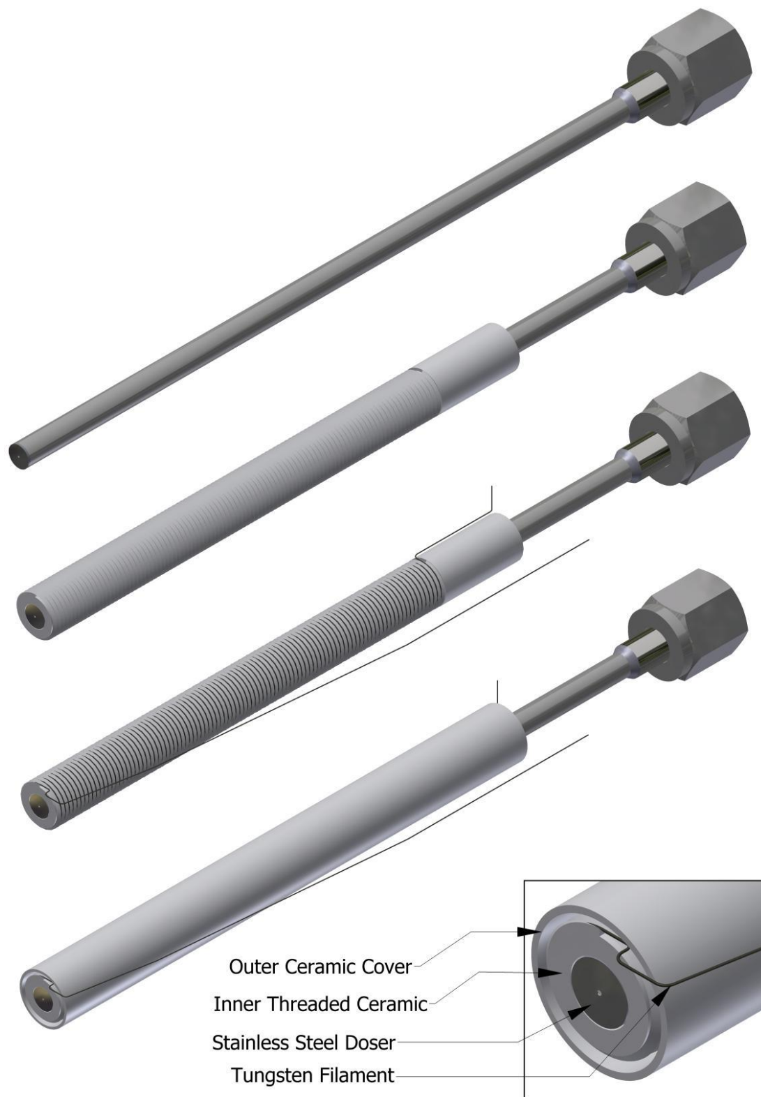
Figure 2.9: a schematic of the three-layer design of the heated effusive molecular beam doser along with a close up view of the nozzle
