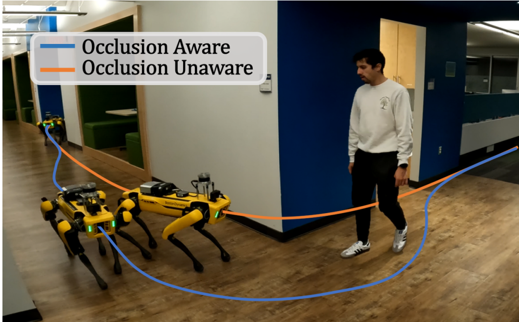
Figure 1.1: Depending on the hallway, the tracking the blue trajectory may be less risky for the robot than tracking the orange trajectory.
