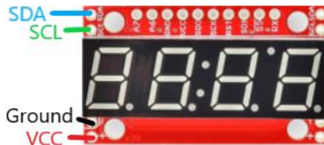
Figure 6: I2C lines for LED Display
