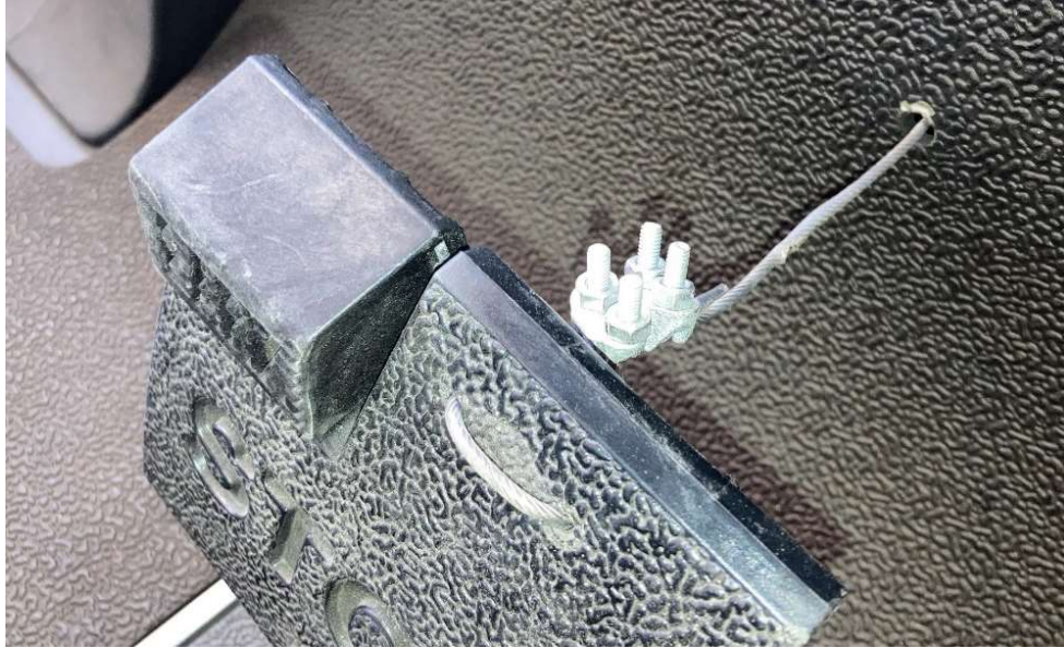
Figure 16. Airline cable secured to the brake pedal
