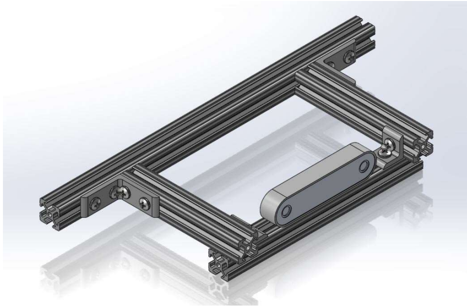
Figure 14: Final design of front-facing camera mount.
