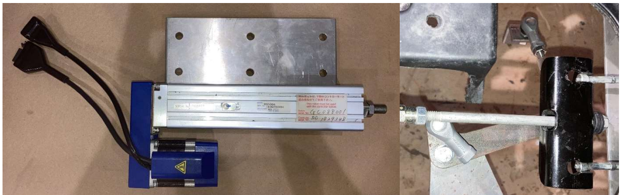
Figure 7: Misumi RSD306 linear actuator and associated braking linkages
