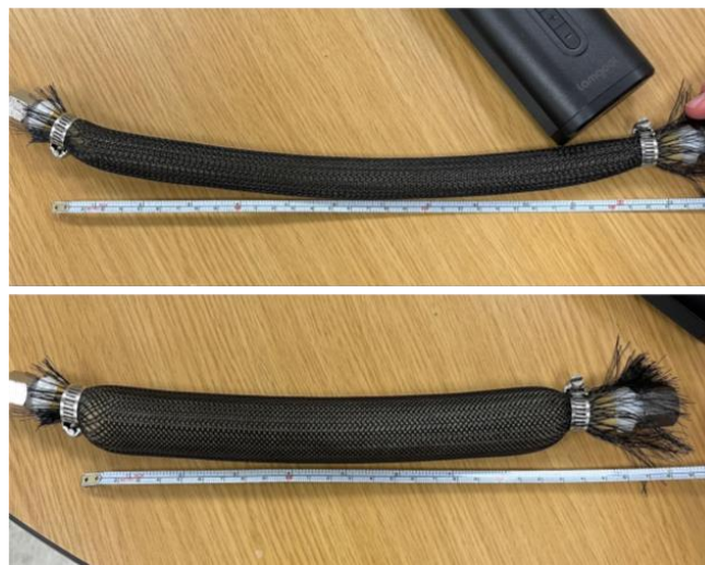
Figure 1. PAM prototype in expanded state (above) and contracted state (below)
