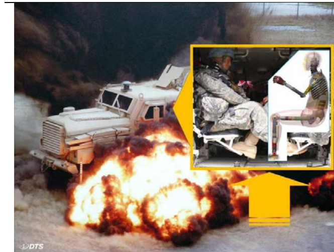
Figure 2. ATD shown experiencing an underbody blast inside an MRAP [11].
