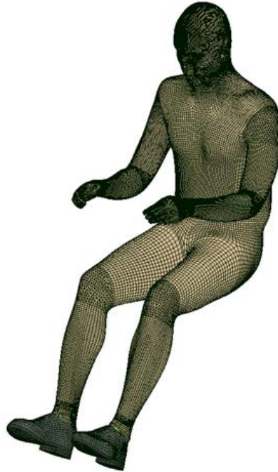
Figure 10. GHBM v4.4 50th percentile male detailed model.
