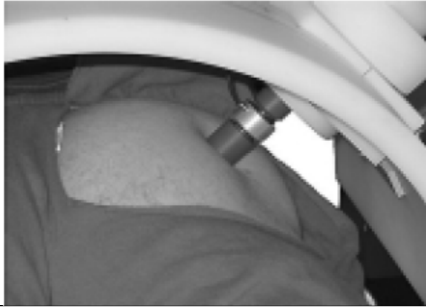
Figure 8. Example of in vivo testing of gluteal tissue through indentation [66]. Figure used with permission (see Chapter 8 for full permission).
