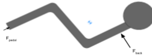
Figure 17: Free body diagram of a rider with reaction forces during pedaling
