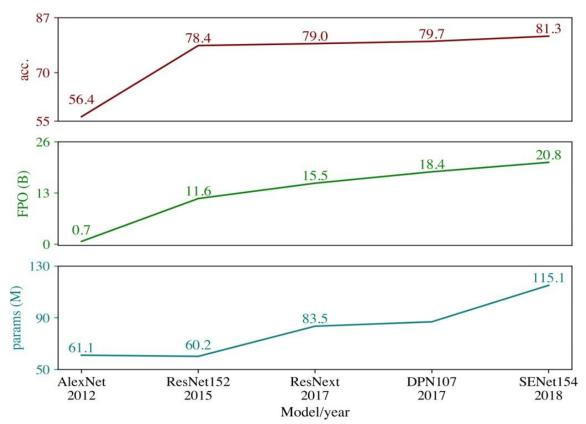
Figure 3: Floating Point Operation(FPO) in billions for different top ImageNet models. This shows how the rate accuracy increases much less steeply than the rate of the FPO increase. (Adapted from 'Green AI' by R. Schwartz, J Dodge, N.Smith, & O. Etzioni. 2019)
