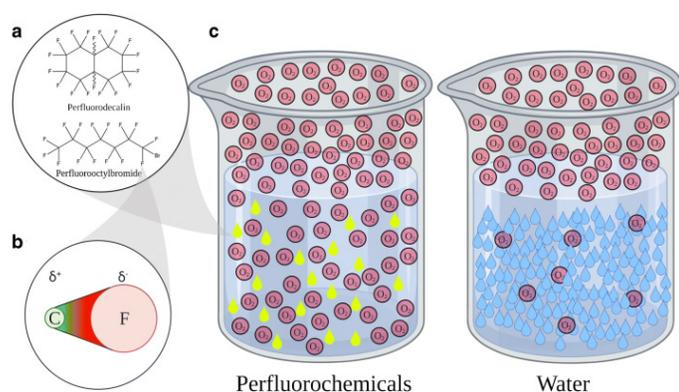
**Fig. 1. Perfluorochemicals, including perfluorocarbons, can dissolve more oxygen than water.** (A) Perfluoro decalin and perfluorooctyl bromide are two examples of common PFCs. (B) Perfluorocarbons have very polarized carbon-fluorine bonds. (C) At the same  $pO_2$ , perfluorocarbons are able to dissolve significantly more oxygen than water due to a low molecular density in solution. Adapted from Jägers et al., 2021.
