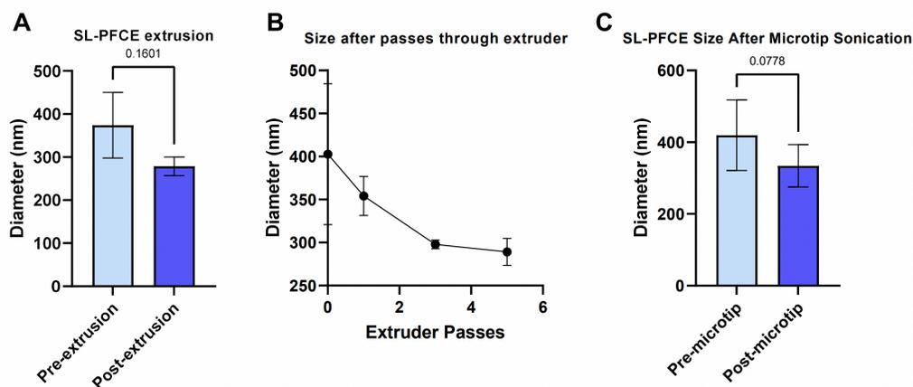
**Fig. 3. Methods of reducing the final size of soy-lecithin-PFCE emulsions.** (A) Extrusion of the soy-lecithin-PFCE emulsions shows a downward trend in diameter ( $n = 3$ ). (B) Extrusions were done with multiple passes through the extruder. Shown is emulsion size after different numbers of passes through the extruder. ( $n = 2$ ). (C) A round of microtip probe sonication following probe sonication with a normal tip shows a downward trend in particle size ( $n = 3$ ).
