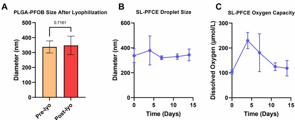
**Fig. 4. Monitoring the stability of synthesized PLGA-PFOB nanoparticles and soy-lecithin-PFCE emulsions over time.** (A) There are no significant changes in PLGA-PFOB nanoparticle diameter with lyophilization ( $n = 3$ ). (B) The diameter of the soy-lecithin-PFCE emulsion droplets measured over a period of 14 days does not change in diameter ( $n = 3$ ). (C) The soy-lecithin-PFCE emulsions maintain oxygen dissolving capabilities over a period of 14 days ( $n = 3$ ).
