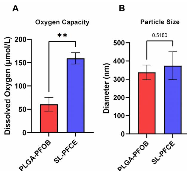
**Fig. 2. Oxygen capacity and particle size of the two formulations.** (A) Soy-lecithin-PFCE emulsions were able to dissolve significantly more oxygen than PLGA-PFOB nanoparticles in solution. \*\* $p < 0.01$  ( $n = 3$ ). (B) Both formulations resulted in similarly sized particles or droplets ( $n = 3$ ).
