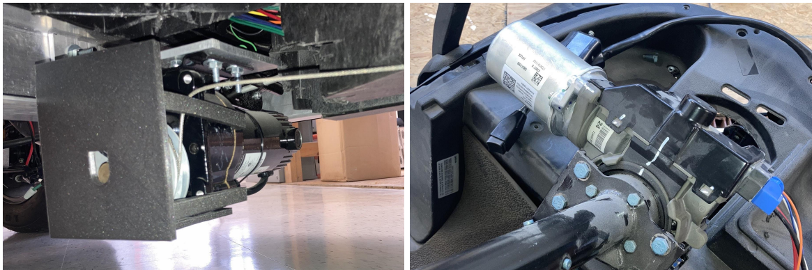
Figure 4: Geared DC motor with attached cable for braking; Nexteer electric power steering system and steering column
