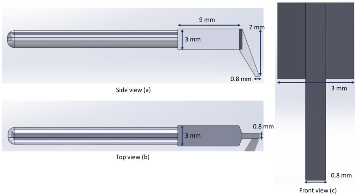
Figure 2.32: 3D-printed tool for plug chip.
