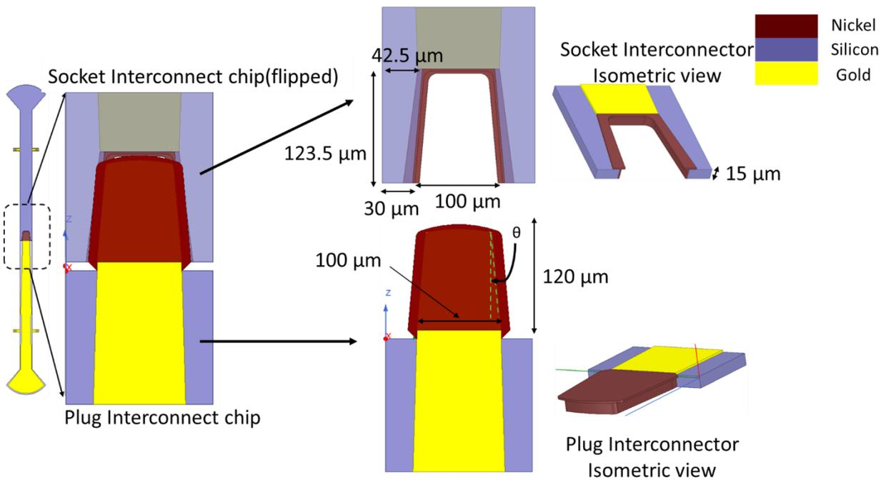
Figure 2.19: Modified chip-to-chip interconnect demonstration.
