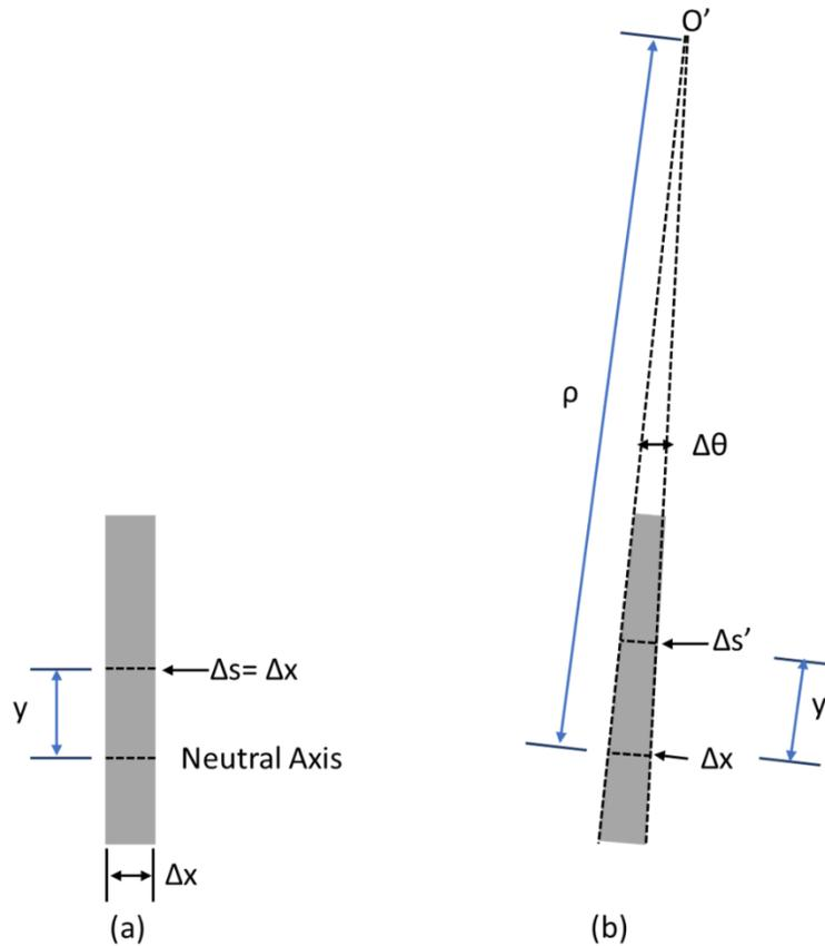
Figure 2.7: Small segments of beam before (a) and after deformed (b).
