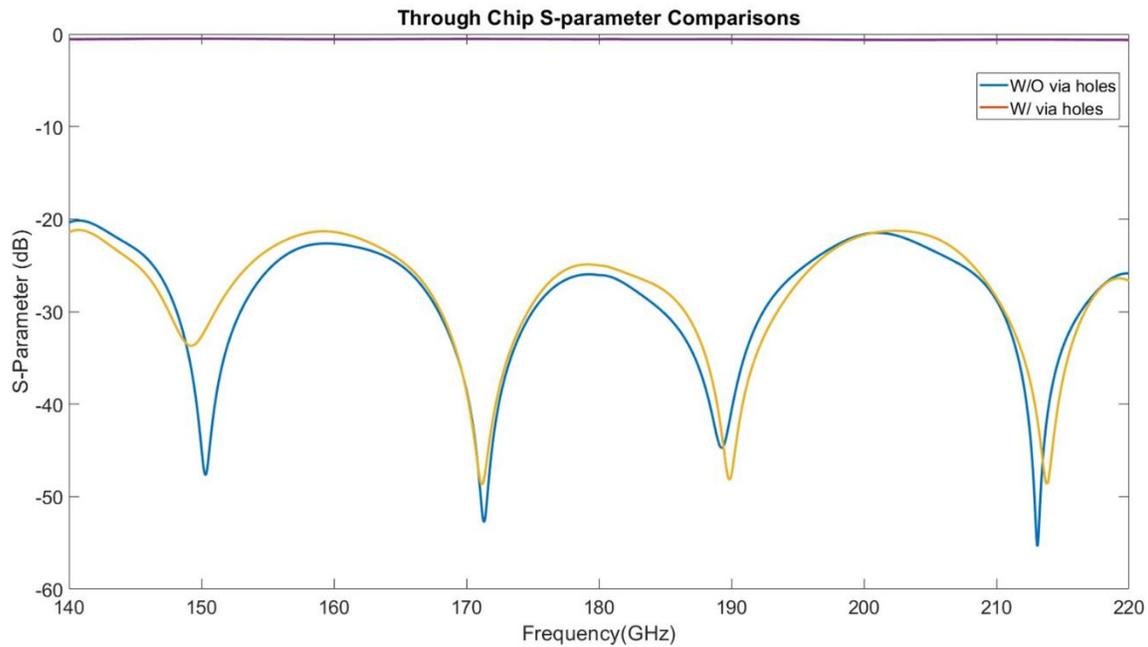
Figure 4.8: Simulation comparison of through chip with and without via holes.
