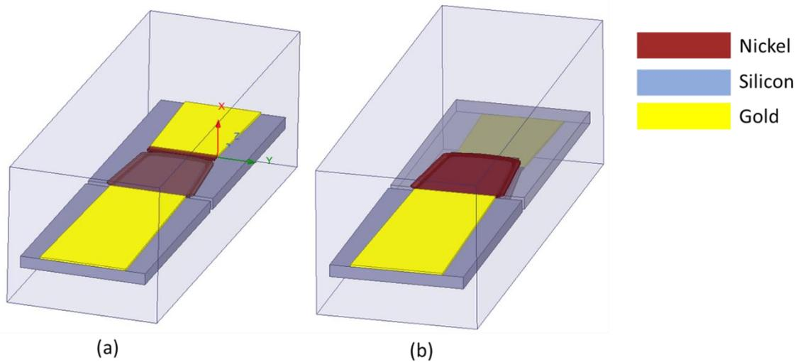
Figure 3.14:(a) Simplified non-flipped interconnect simulation (b) Simplified non-flipped interconnect simulation.
