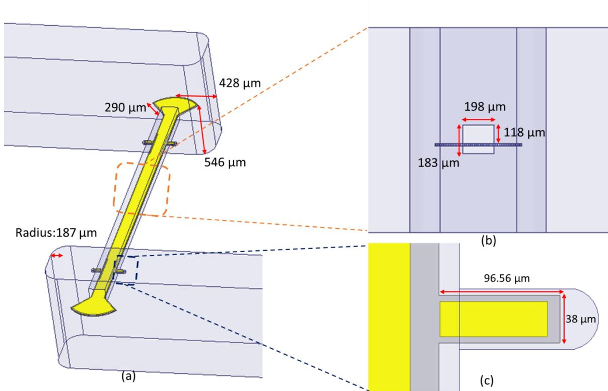
Figure 3.4: (a) Interconnects inside waveguide housing (b) Interconnects inside the RF Channel (c) clamp structure.
