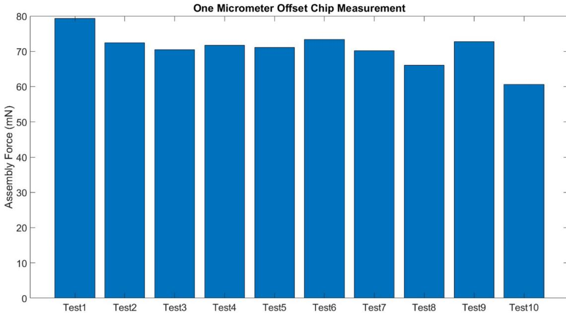
Figure 2.36: 1 $\mu$ m offset chip assembly force measure results.
