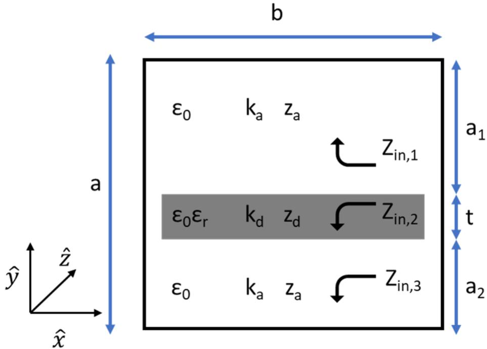
Figure 3.2: Cross section view and transmission line model of coaxial line channel.
