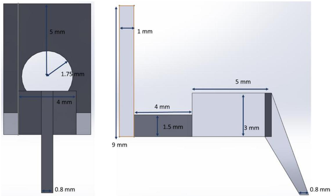
Figure 2.30: 3D-printed tool for socket chip.
