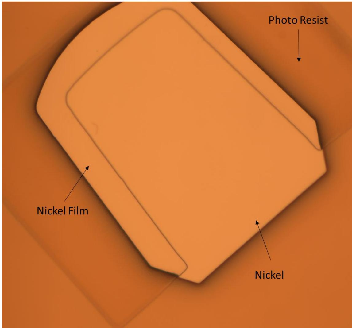
Figure B. 3:Photolithography of AZ-4330 in Via hole.
