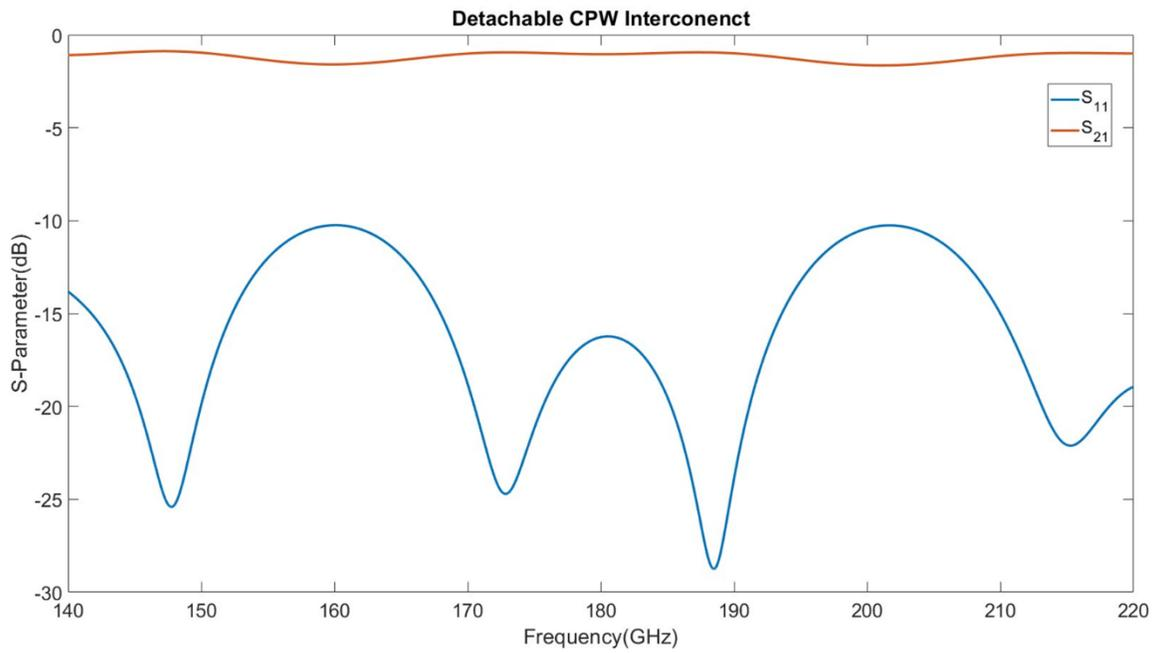
Figure 4.11: Simulation results of CPW line with interconnect.
