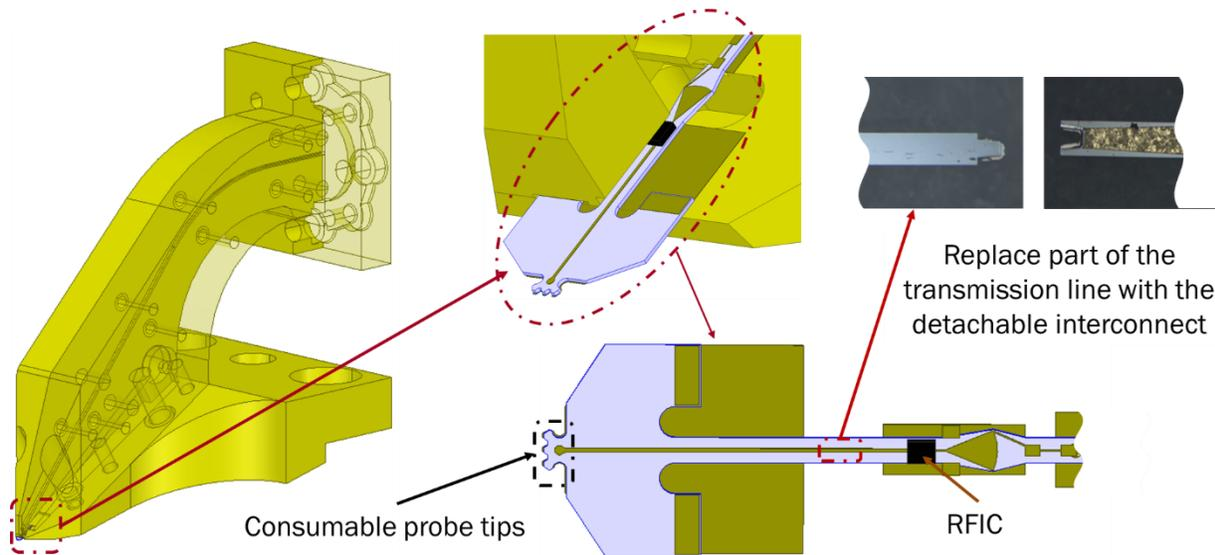
*Figure 1.10: Micro-machined on-wafer probe station, probe chips and chip-to-chip interconnects.*
