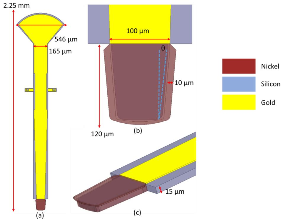
Figure 3.9:(a) Plug chip layout (b) Interconnector part (c) Isometric view of interconnector.
