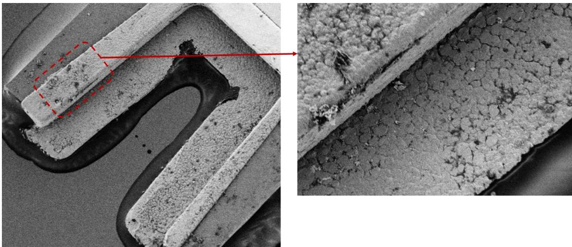
Figure 2.50: SEM pictures of broken socket chips (Test3).
