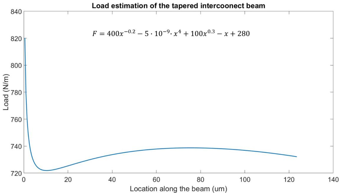
Figure 2.22: Modified Chip-to-chip interconnects load estimation.
