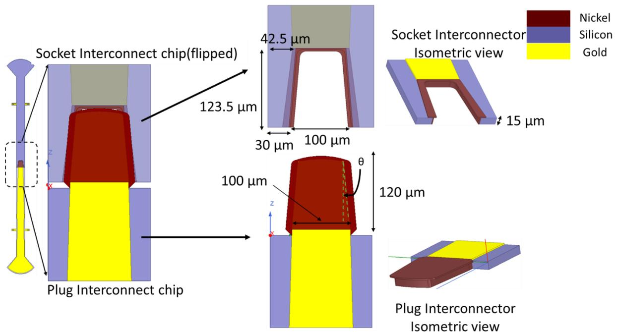
Figure 3.3: Detachable chip-to-chip interconnect demonstration.
