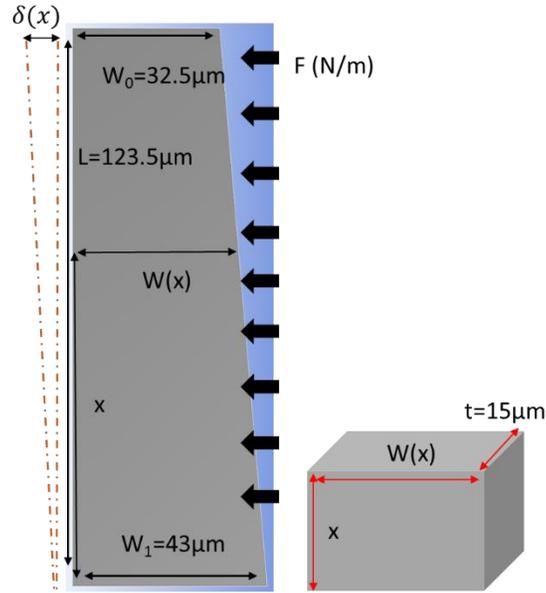
Figure 2.20: Non-prismatic beam applied with uniform load.
