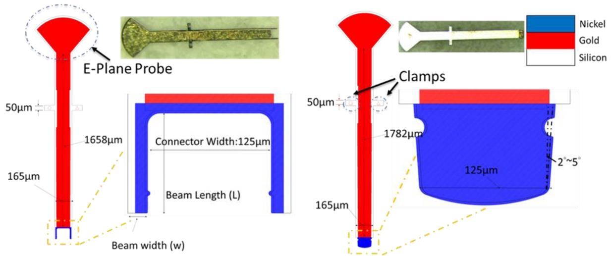
Figure 2.14: Chip-to-chip detachable socket and plug chips prototype.
