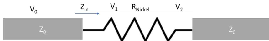
Figure 2.43: Nickel interface resistance and insertion loss model.
