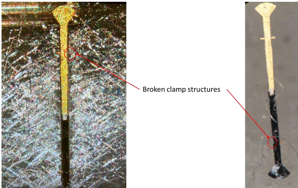
Figure 4.4: Images of broken clamp structures during assembly process.
