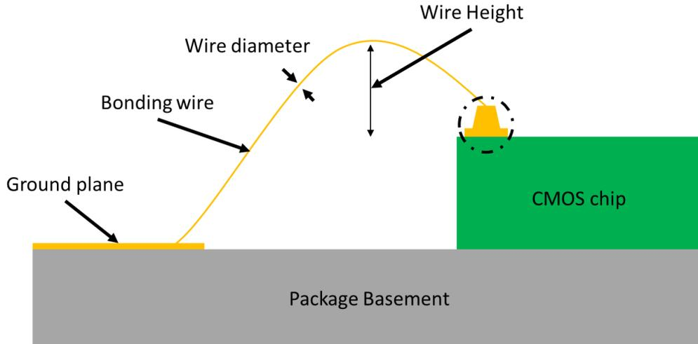
*Figure 1.4: Typical bond wire connection.*
