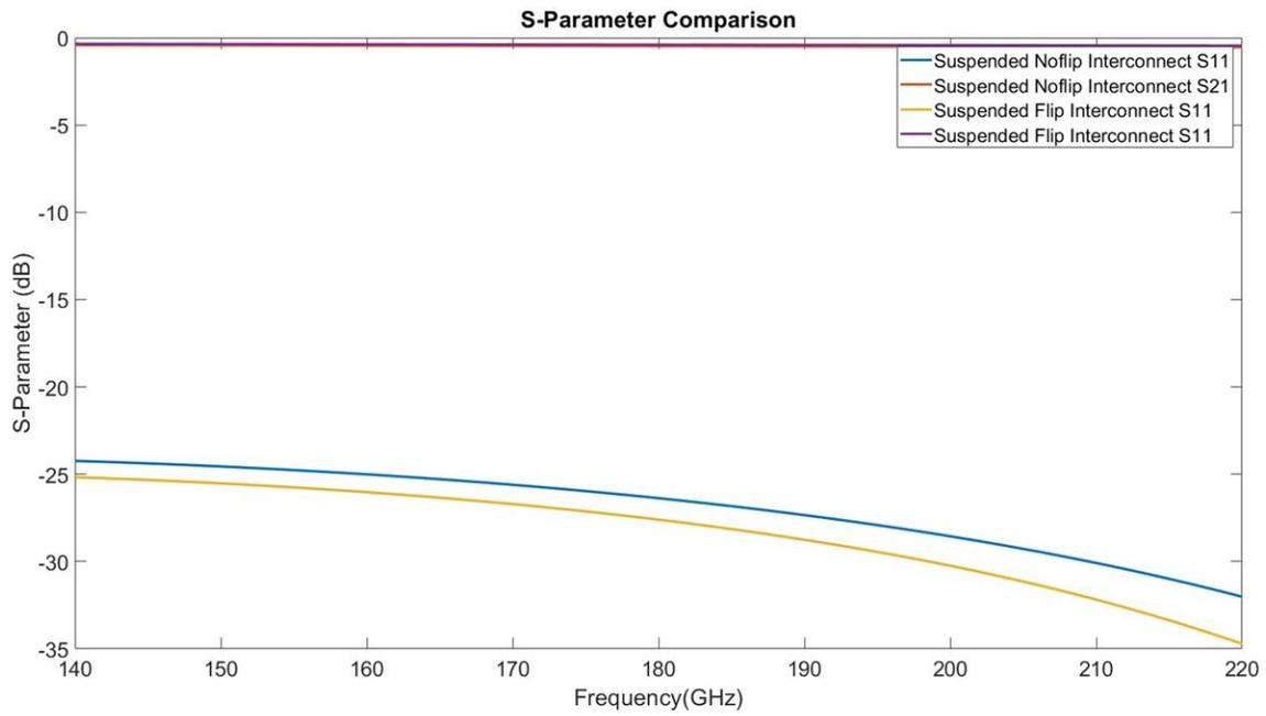
Figure 3.16: Simulation results of simplified flipped and non-flipped interconnector.
