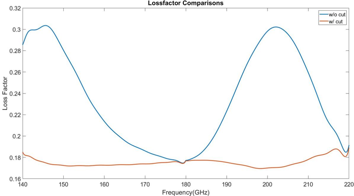
Figure 3.8: Through chip loss factor simulation comparison.
