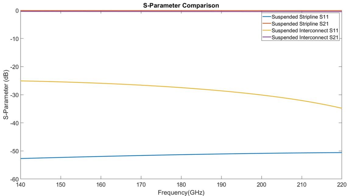
Figure 3.21:S-parameter comparison of suspended stripline and interconnect.
