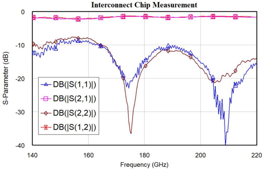
Figure 3.28: chip-to-chip interconnect measured results.
