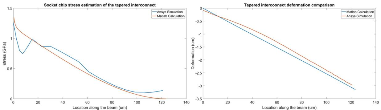
Figure 2.23: Tapered Chip-to-chip interconnects stress and deformation comparison.
