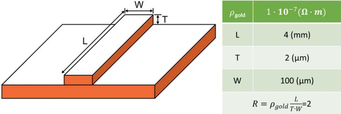
Figure 2.42:Gold trace resistance calculation.
