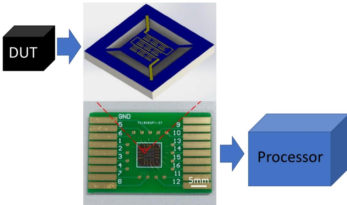
Figure 1.1: Terahertz detector array and detection system [12].
