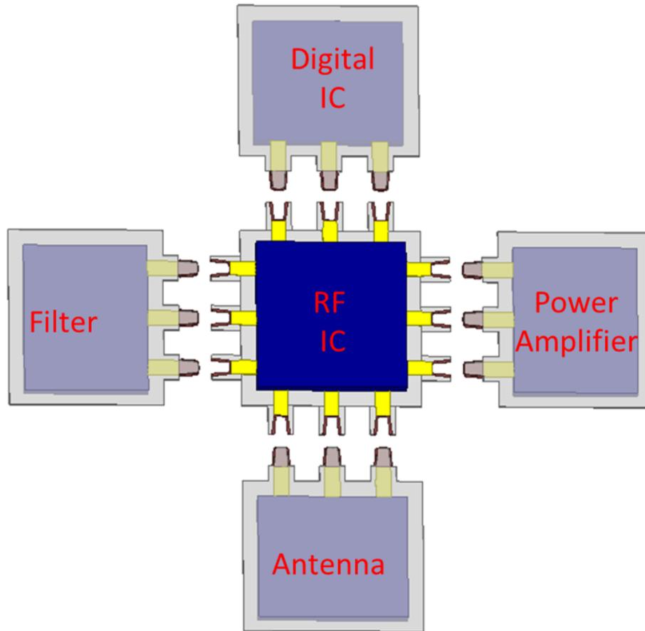
Figure 4.9: Chip-to-chip interconnect on CPW mode and system concept.
