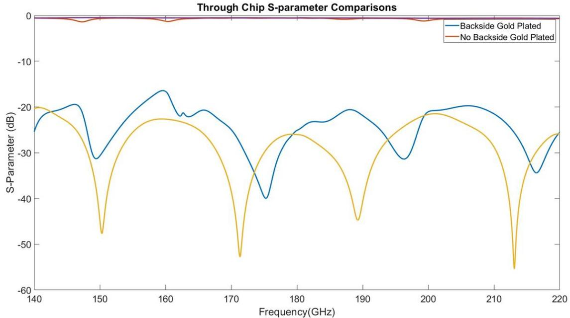
Figure 4.6: Through chip simulation comparison.
