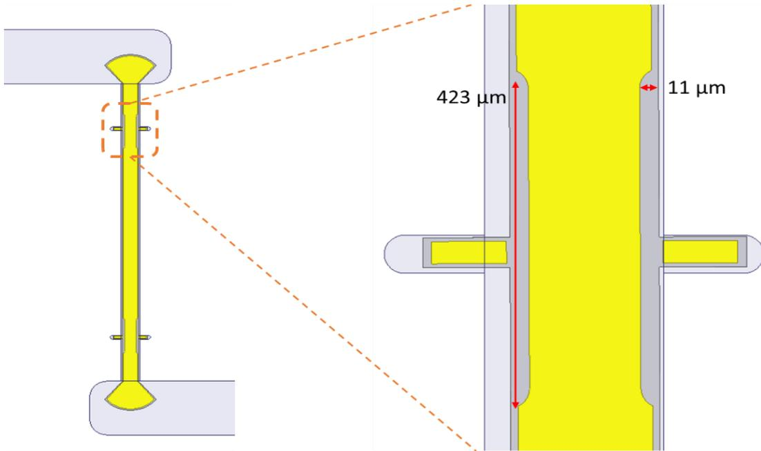
Figure 3.7: Interconnects inside waveguide housing and the clamp compensation structure.
