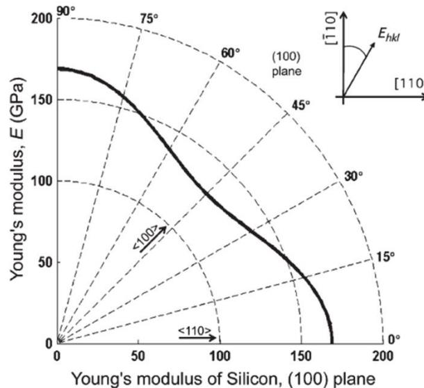
Figure 2.10: Values of Young's Modulus versus orientation in silicon [110] plane [42].
