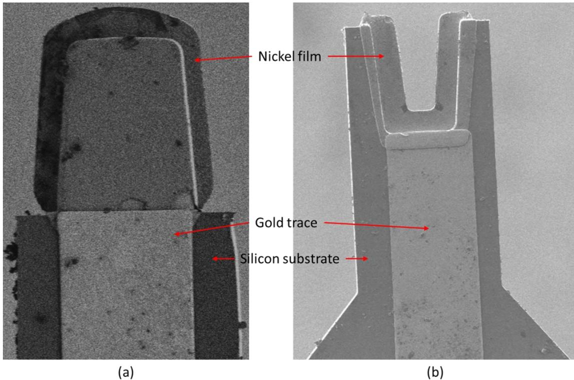
Figure 2.27: SEM images of (a) Plug chip (b) Socket chip
