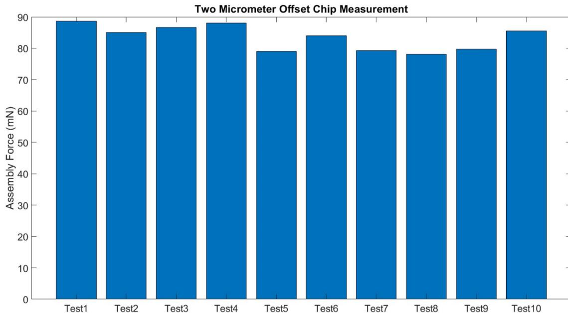
Figure 2.35: 2  $\mu\text{m}$  offset chip assembly force measure results.
