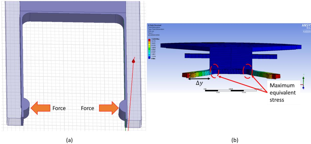
Figure 2.15: Ansys Mechanics simulation layout (a) and results (b)
