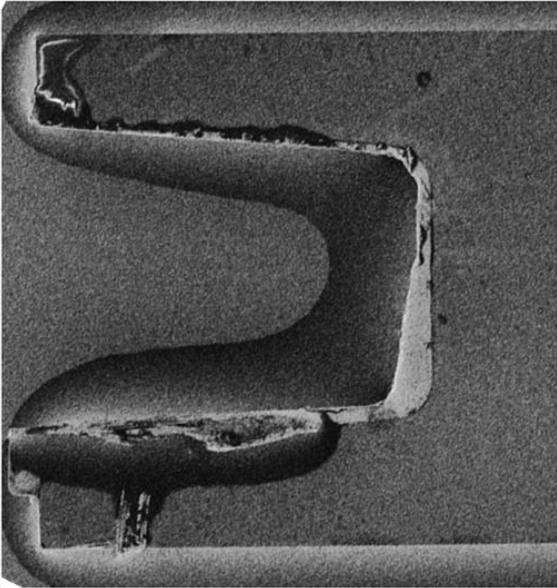
Figure 2.52:SEM pictures of 1  $\mu\text{m}$  offset socket chips after 100 times of lifetime measurement.
