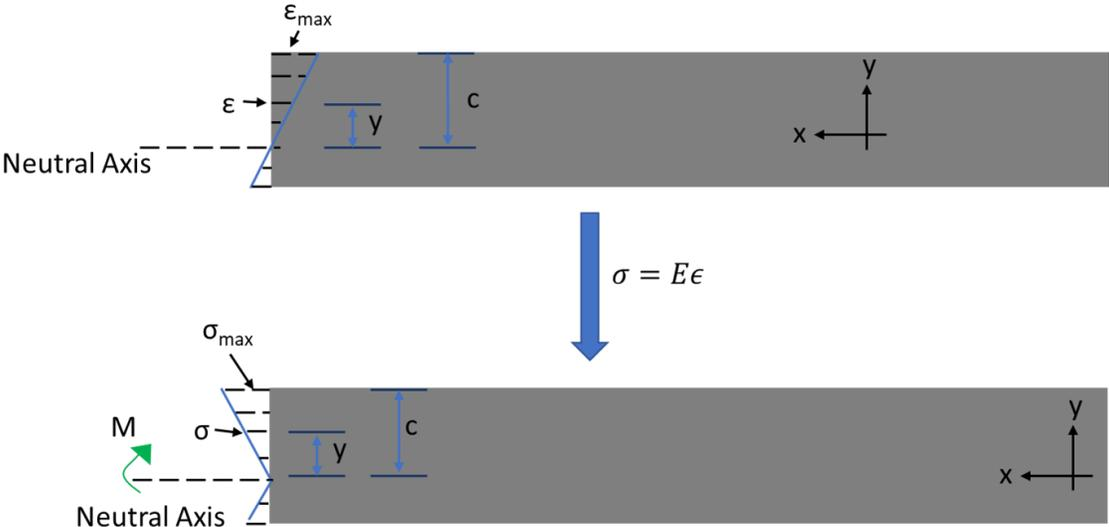
Figure 2.8: Strain and stress beam diagram.
