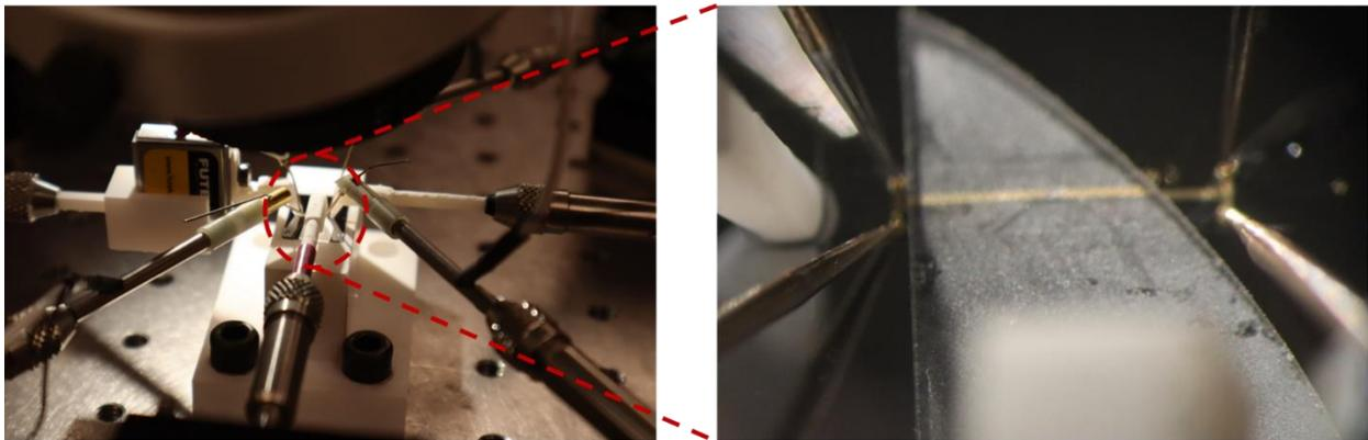
Figure 2.38: Contact resistance and pull test setup.
