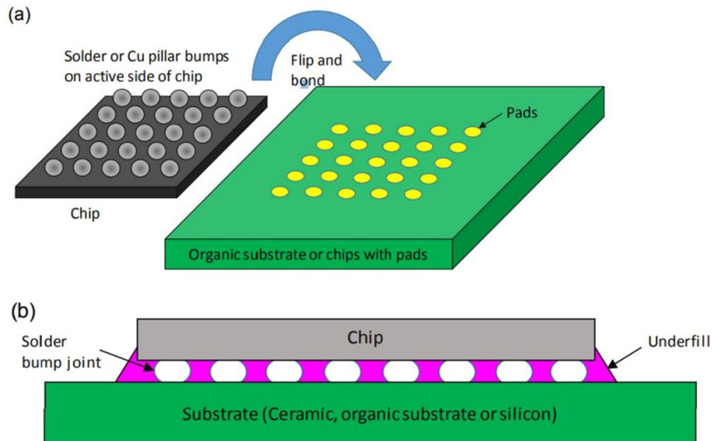
Figure 1.5: Demonstration of C4 bonding and cross section illustration of bonding stacks [33].
