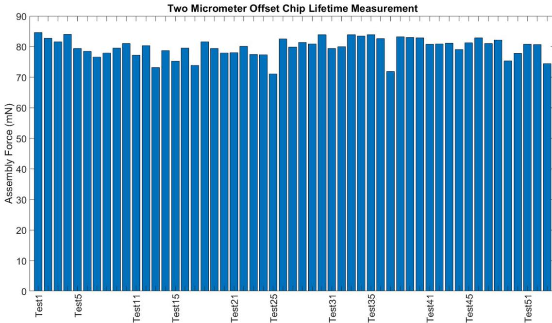
Figure 2.49: Third lifetime test of 2  $\mu\text{m}$  offset chip measurement.
