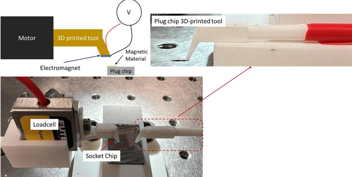
Figure 4.3: Modified assembly and disassembly force measurement.
