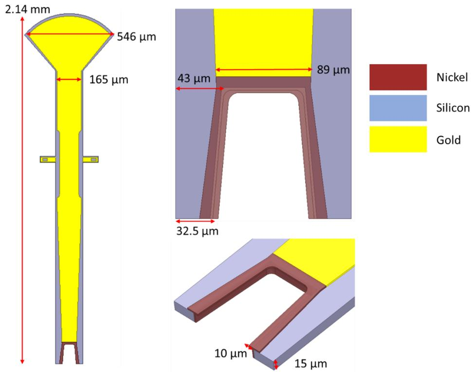
Figure 3.10:(a) Socket chip layout (b) Interconnector part (c) Isometric view of interconnector
