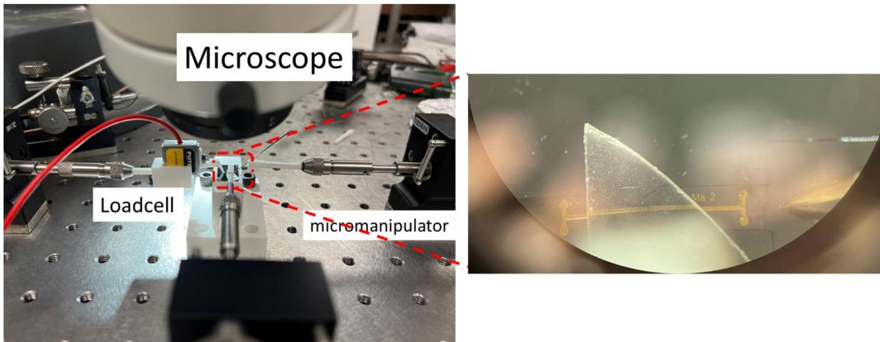
Figure 2.37: Disassembly full measurement.
