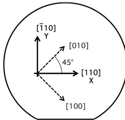
Figure 2.9: Direction of axes in [110] wafer [42].
