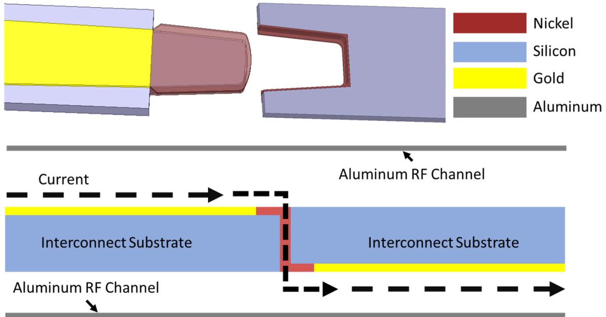
Figure 3.13: Chip to chip interconnect flipped assembly and current flow
