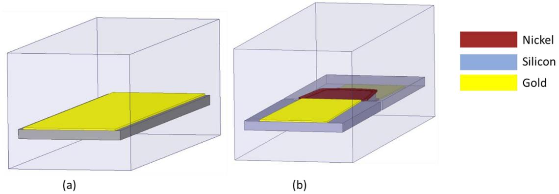
Figure 3.20:(a) Suspended stripline inside RF channel (b) Suspended interconnect inside RF channel.
