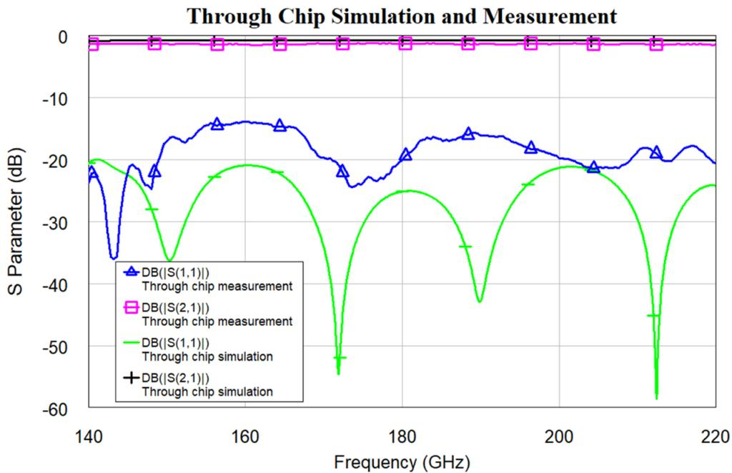
Figure 3.25: Simulation and measurement comparison of through chip.
