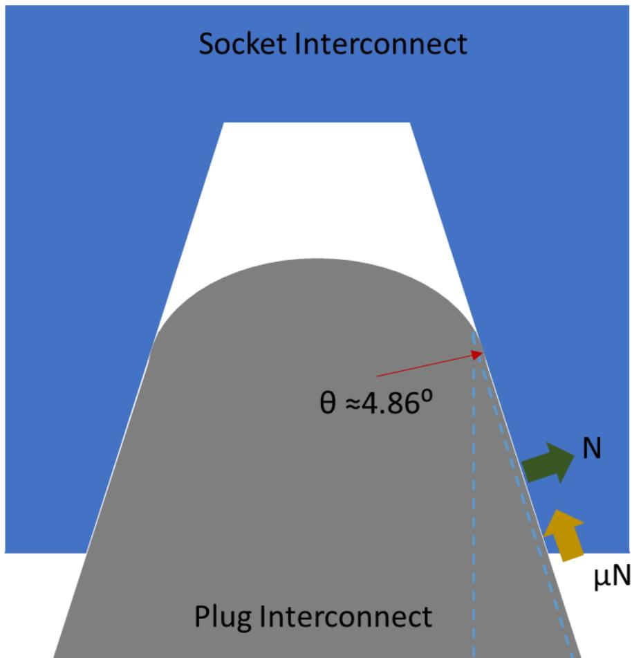
Figure 2.25: Disassembly force analysis
