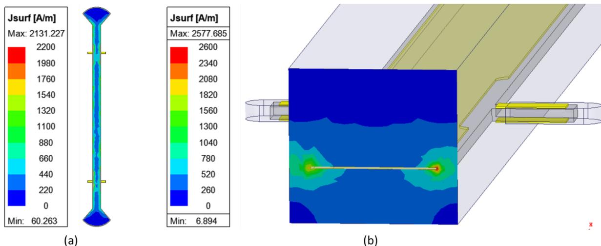
Figure 3.5:(a) Through chip current distribution (b) cross section simulation of through chip current distribution.
