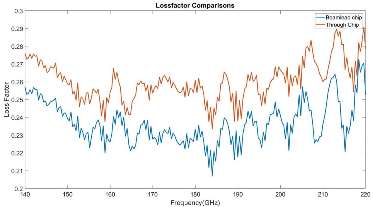
Figure 3.35: Lossfactor comparison of beam lead chip and through chip.
