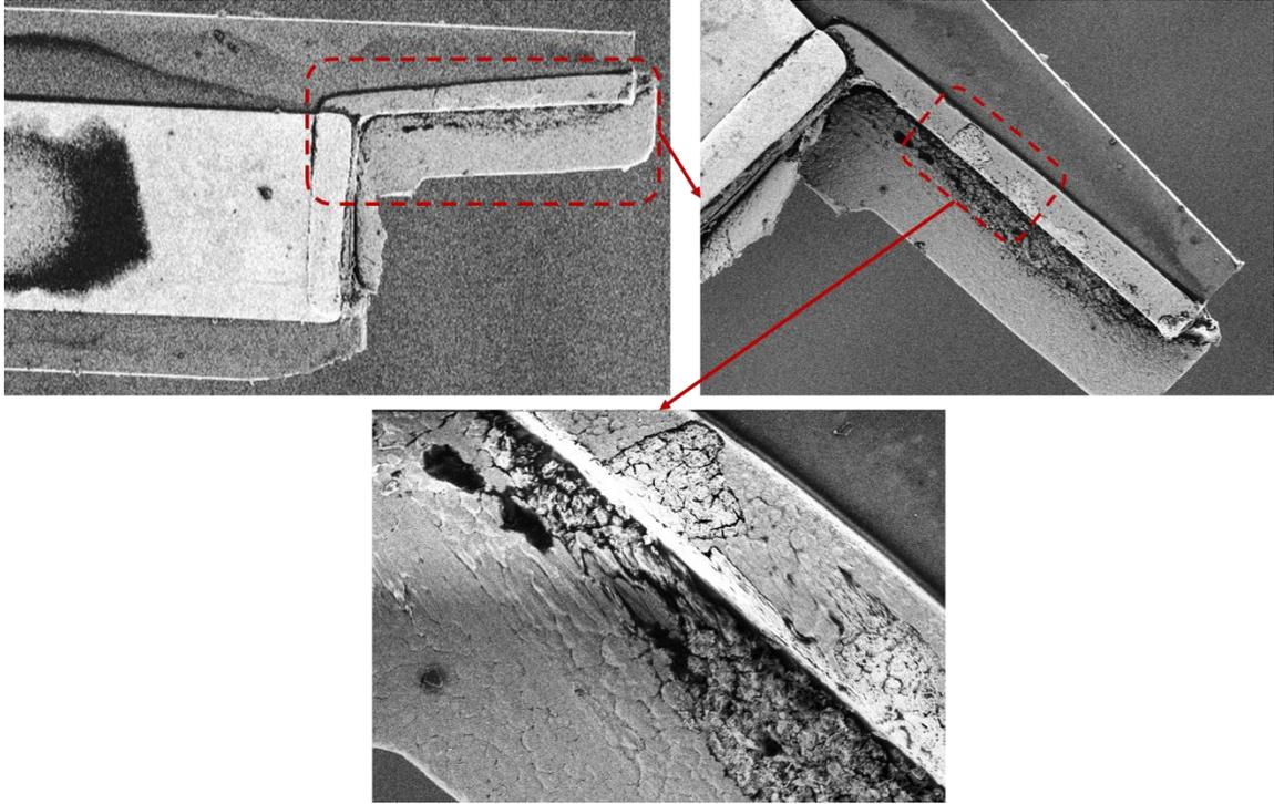
*Figure 2.47: SEM pictures of broken socket chips (Test2).*
