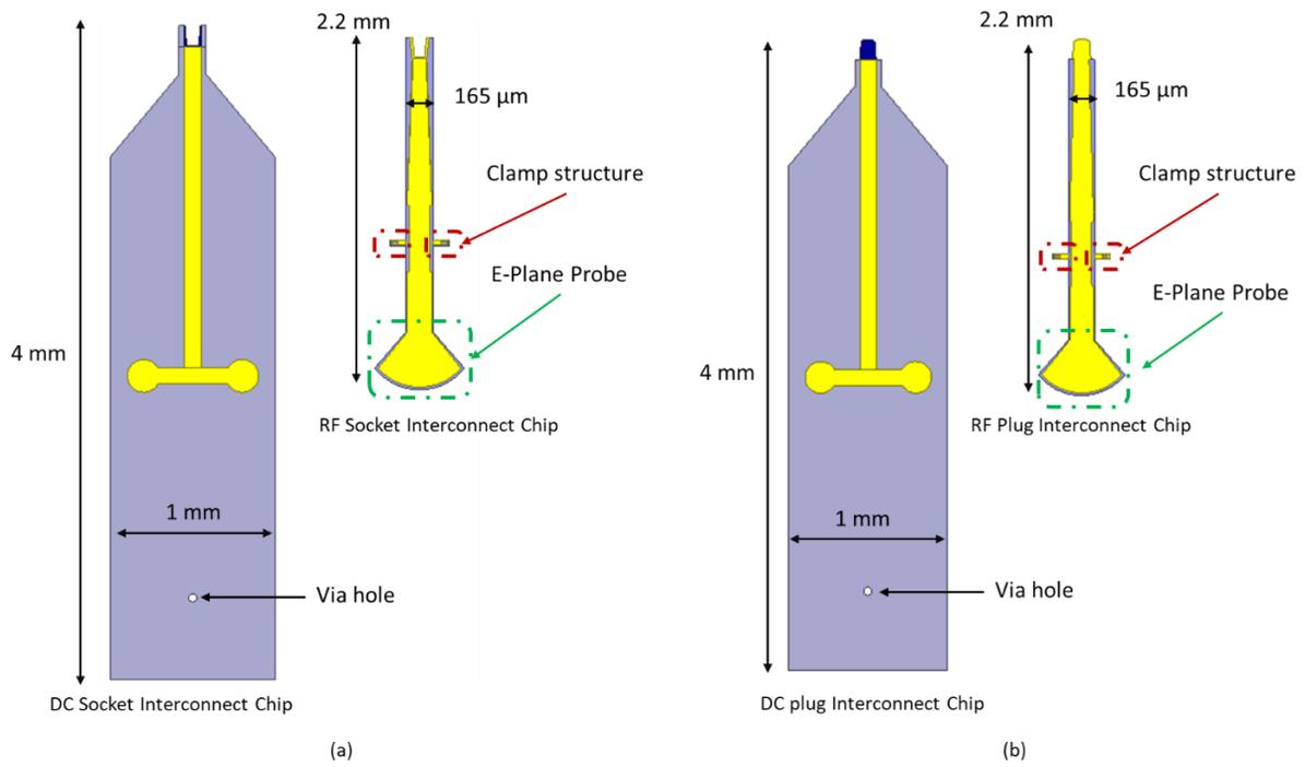
Figure 2.28: Size comparison of DC interconnect chip and RF interconnect chip (a) Socket chip (b) Plug chip
