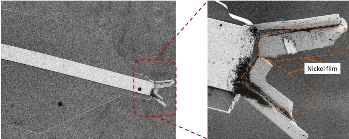
Figure 2.46: SEM pictures of broken socket chips (Test1).
