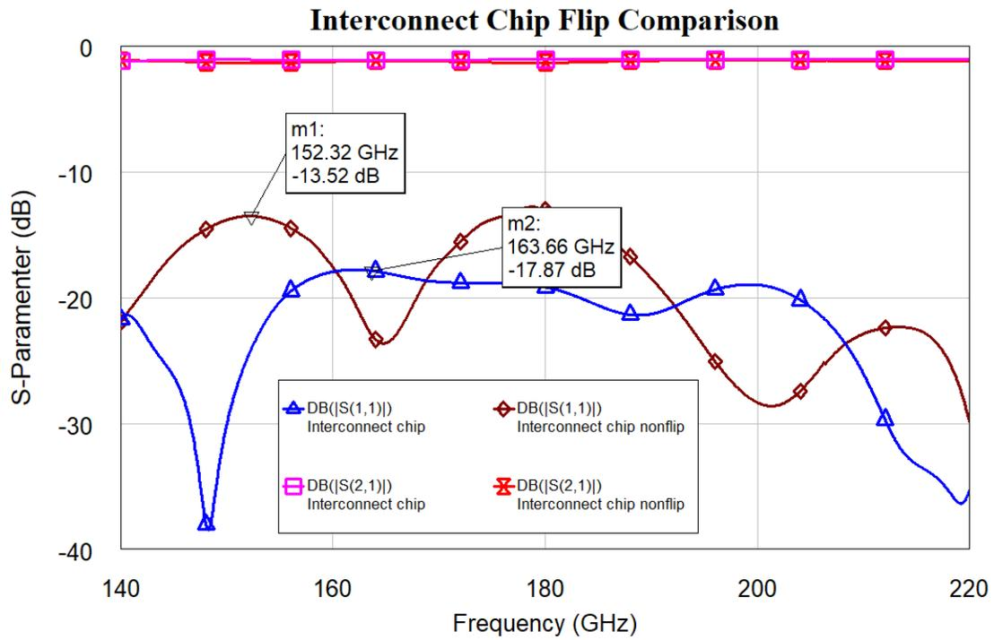
Figure 3.12: Interconnect chip simulation with and without flipped.
