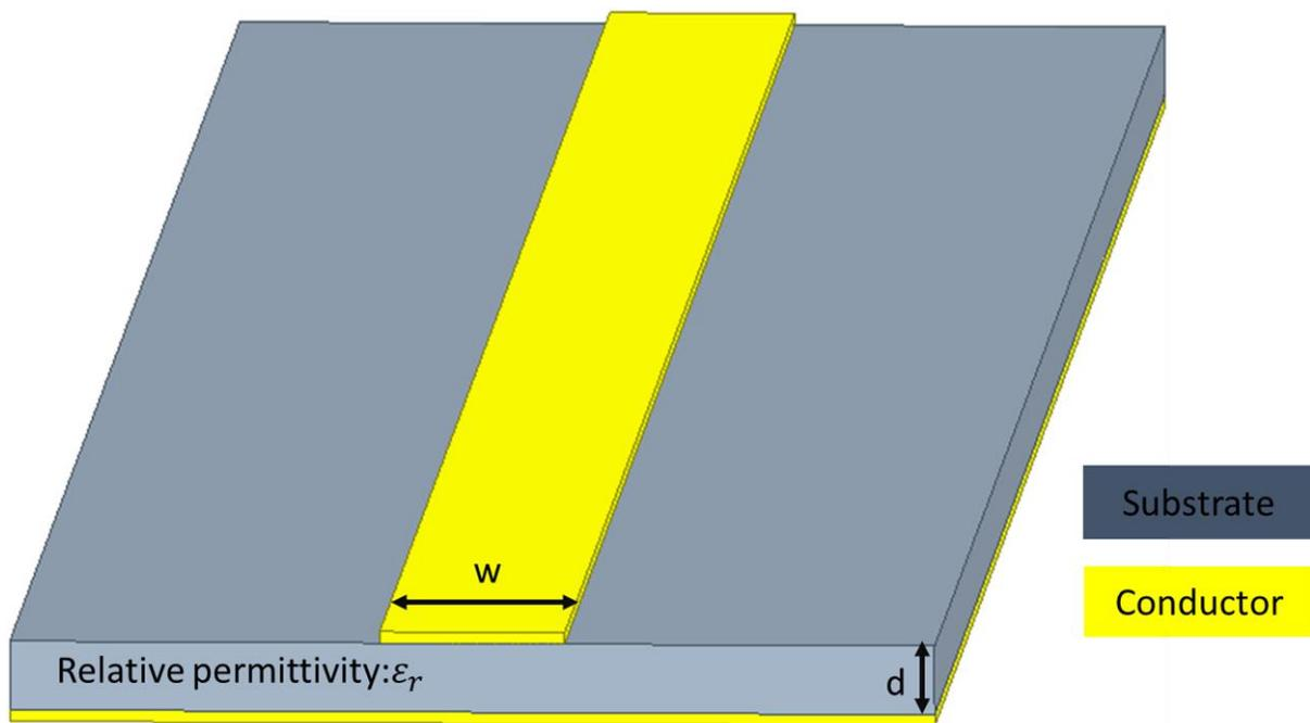
Figure 3.1: Geometry of a Microstrip line
