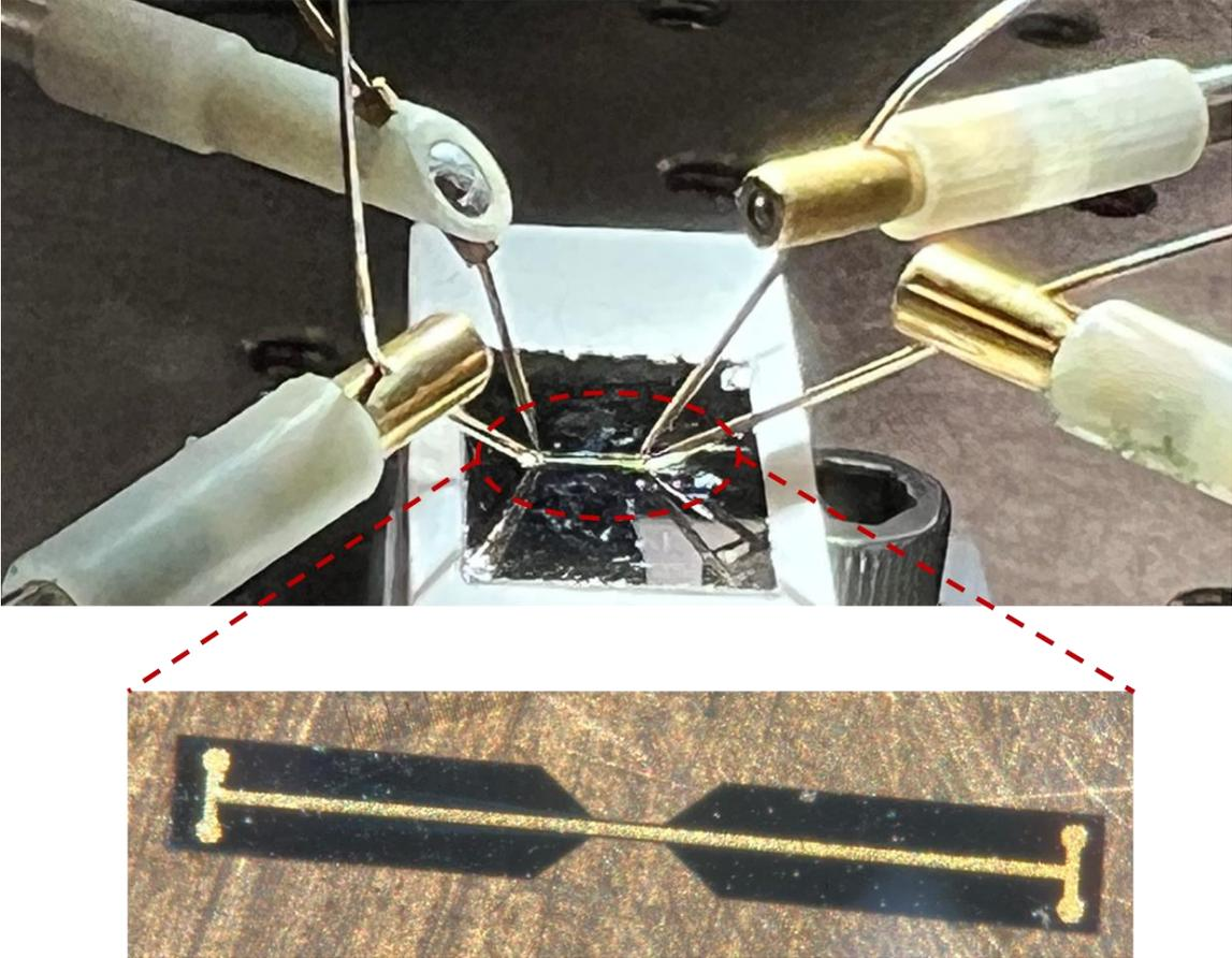
Figure 2.41:Four point measurement of gold trace resistance.
