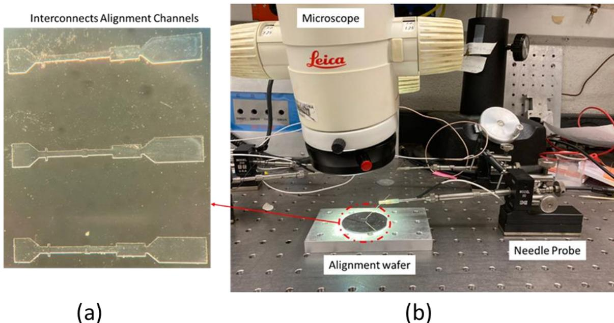
Figure 2.16: Chip-to-chip interconnect prototype alignment wafer (a) and assembly setup (b).
