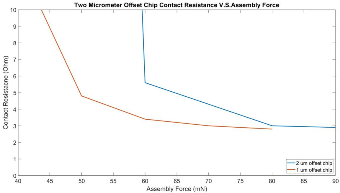
Figure 2.48: contact resistance versus assembly force.
