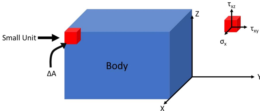
Figure 2.3: Concept of normal stress and shear stress.
