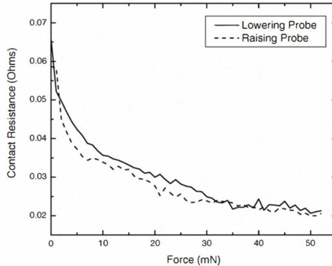
Figure 2.12: Gold to gold contact force vs. contact resistance [43].
