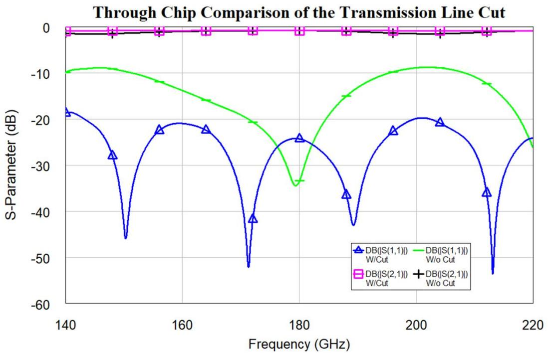
Figure 3.6: Simulation of through chip with and without cut structure.
