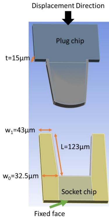
Figure 2.24: Ansys simulation of tapered interconnect assembly.
