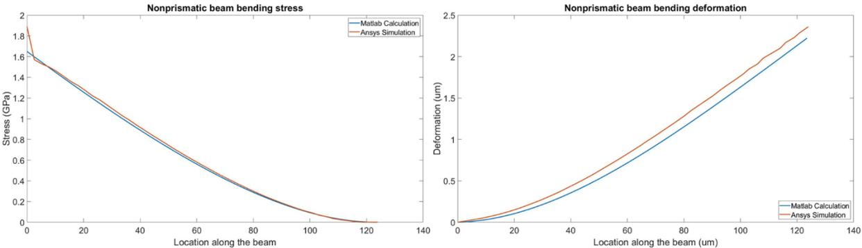
Figure 2.21: Non-prismatic beam stress and deformation comparison.
