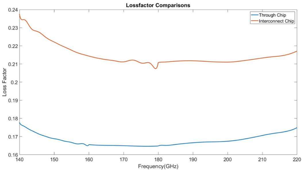
Figure 3.18: Loss factor comparison between through chip and interconnect chip.
