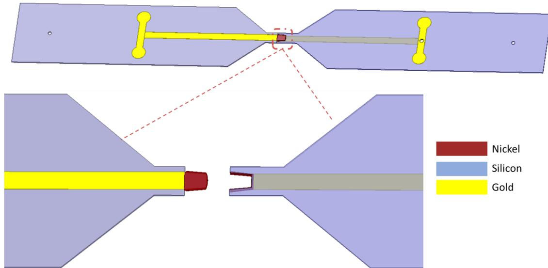
Figure 4.2: Modified DC chip with flipped assembly.
