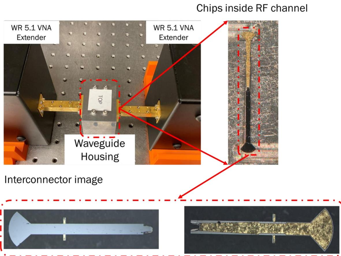
Figure 3.24: Chip-to-chip interconnect waveguide housing and interconnect chips.
