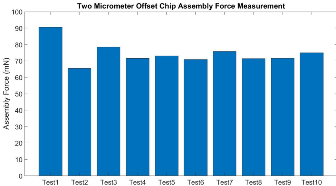
Figure 2.39: Assembly Force measurement for 2  $\mu\text{m}$  offset.
