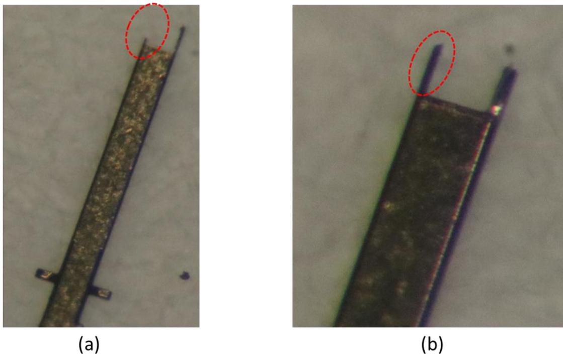
Figure 2.17: Detachable chip-to-chip interconnect prototype socket chips fail examples (a) broken arms (b) cracked arms
