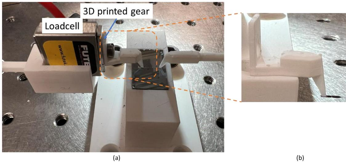
Figure 2.29: (a) Assembly force measurement setup and (b) 3D printed tool for socket chip.
