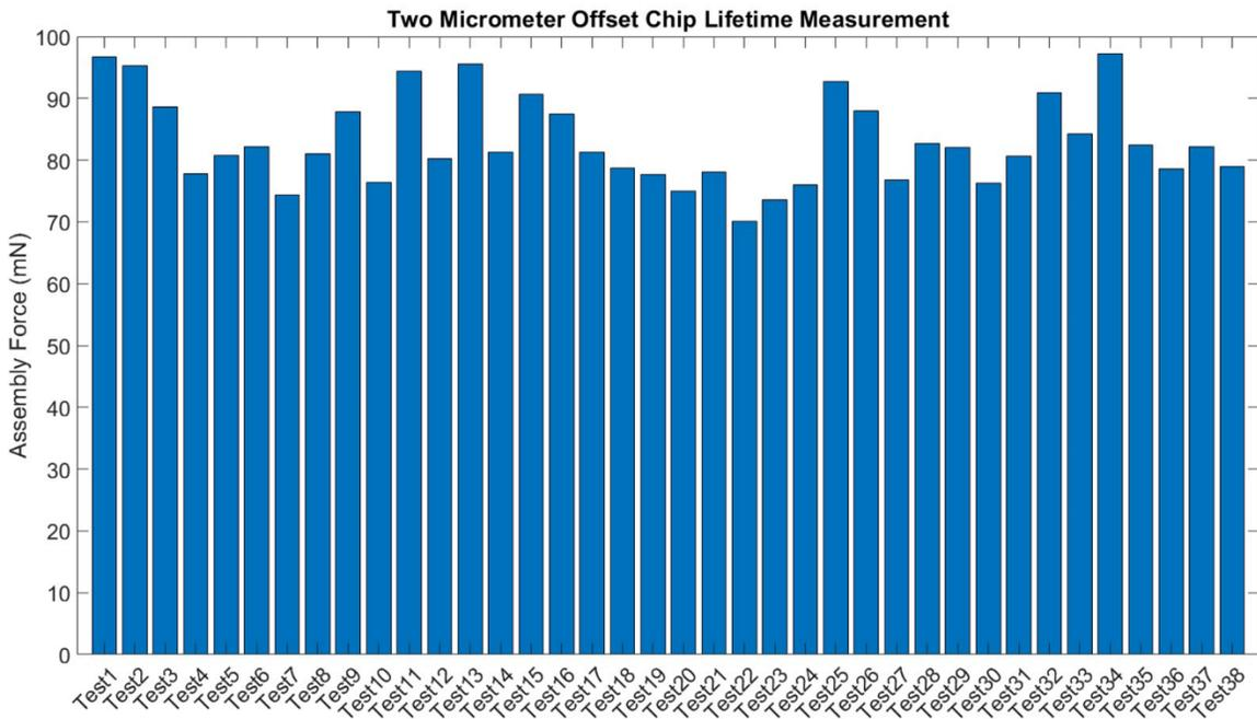
Figure 2.45: Second lifetime test of 2  $\mu\text{m}$  offset chip measurement.
