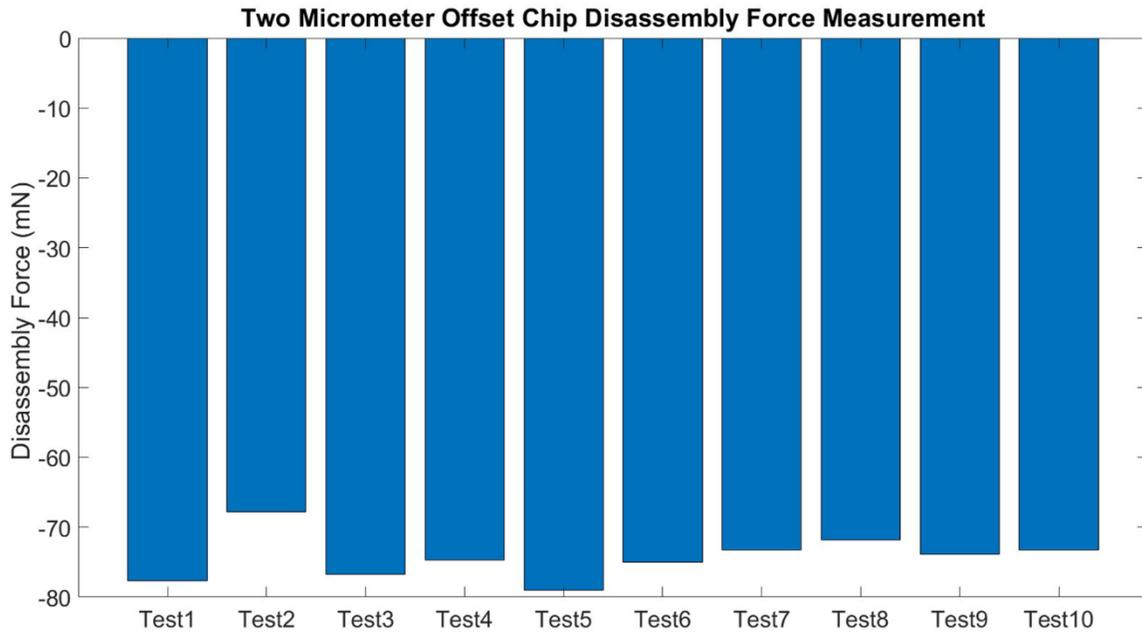
Figure 2.40: Disassembly Force measurement for 2 μm offset.
