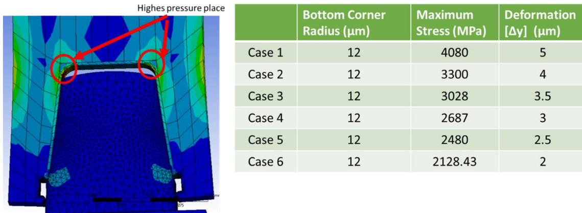
Figure 2.26:(a) Ansys Mechanical layout (b) Ansys Mechanical stress simulation summarizes.
