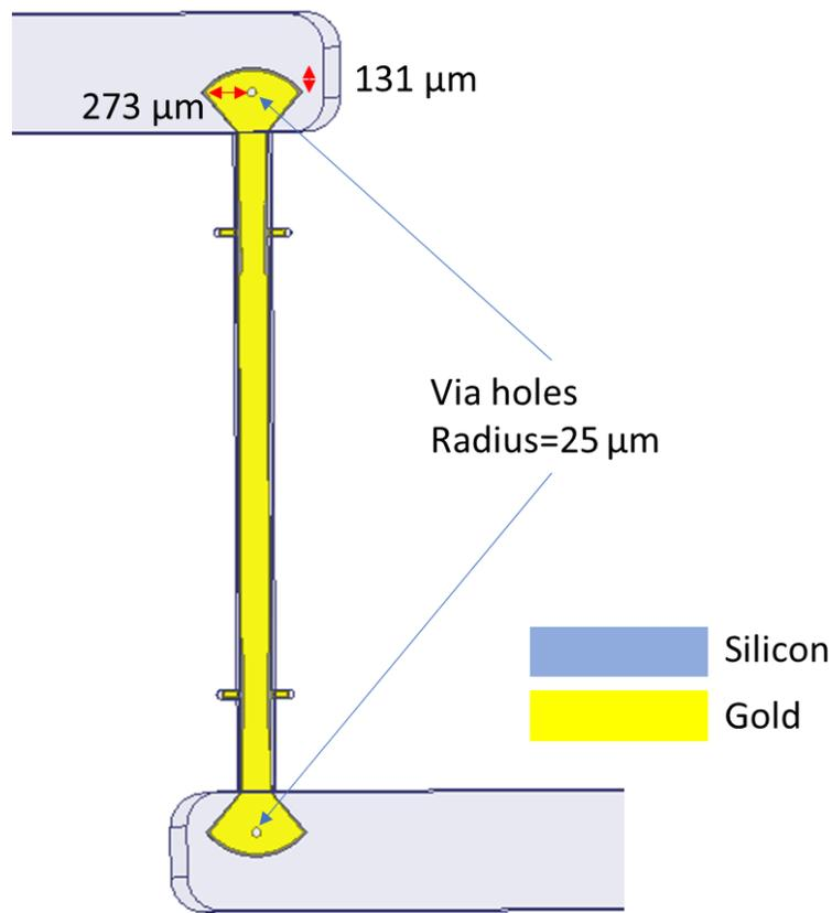
Figure 4.7: Through chip with via holes on the E-plane probes.
