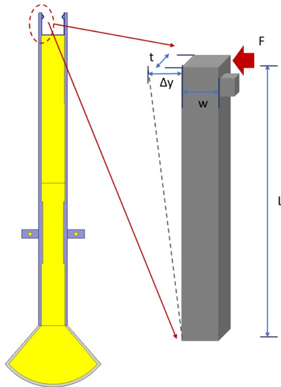
Figure 2.13: Chip-to-chip detachable socket chip and interconnect arm structure.
