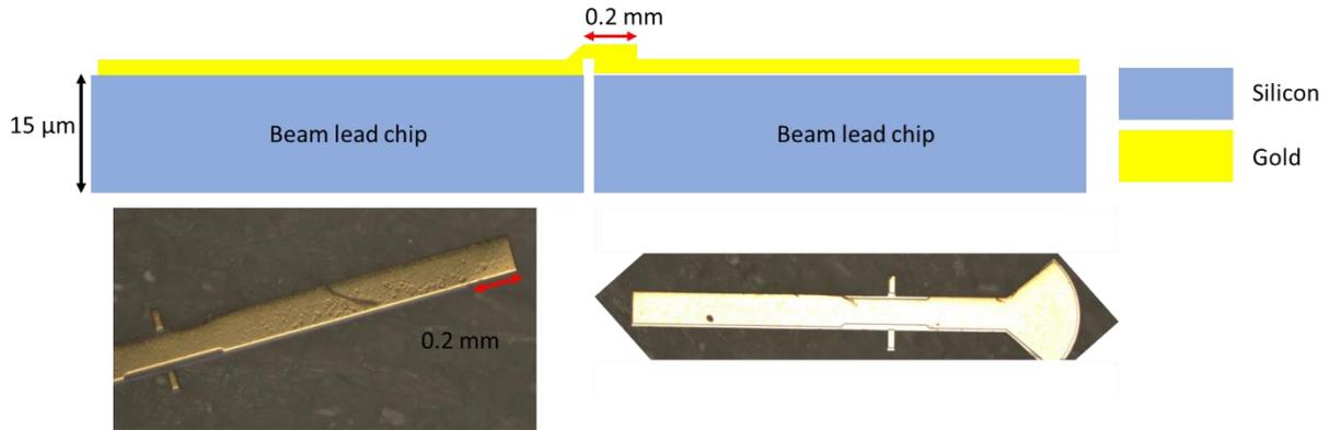
Figure 3.32: Beam lead chip conception demonstration.
