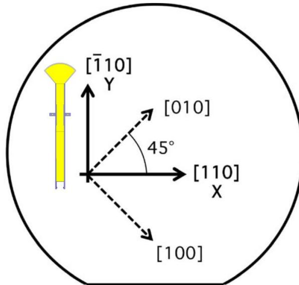
Figure 2.11: Prototype interconnect placement versus orientation [42].
