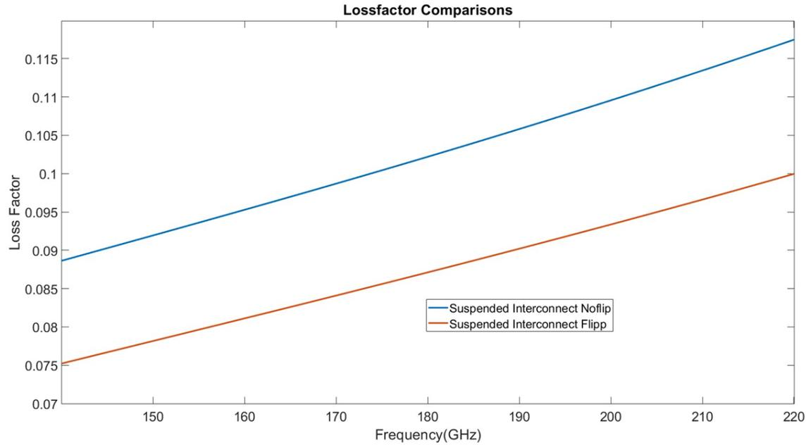
Figure 3.15: Lossfactor Simulation of simplified flipped and non-flipped interconnectors.
