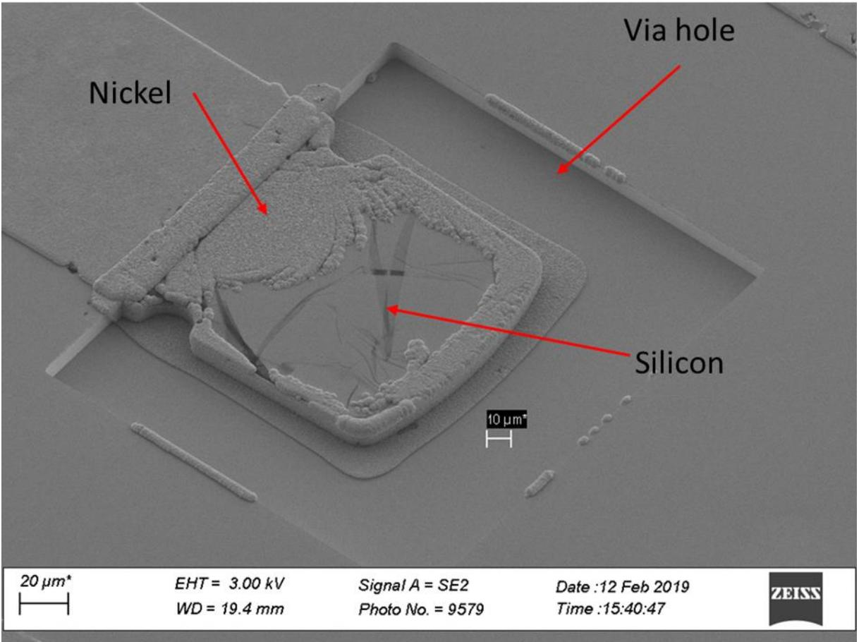
Figure B. 1: Nickel electroplated on Ti/Au Seed-layer.
