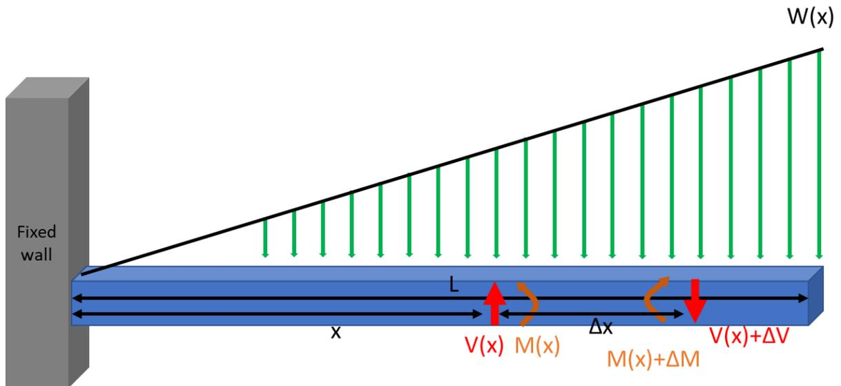
Figure 2.4: Fix cantilever beam diagram.
