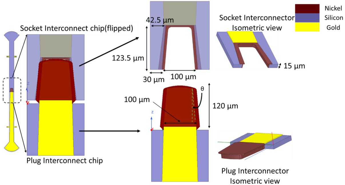
Figure 3.17: Comprehensive simulation of chip-to-chip interconnect.
