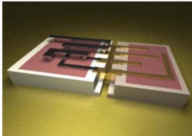
*Figure 1.6: Demonstration of two chips connected by quick packaging [39].*
