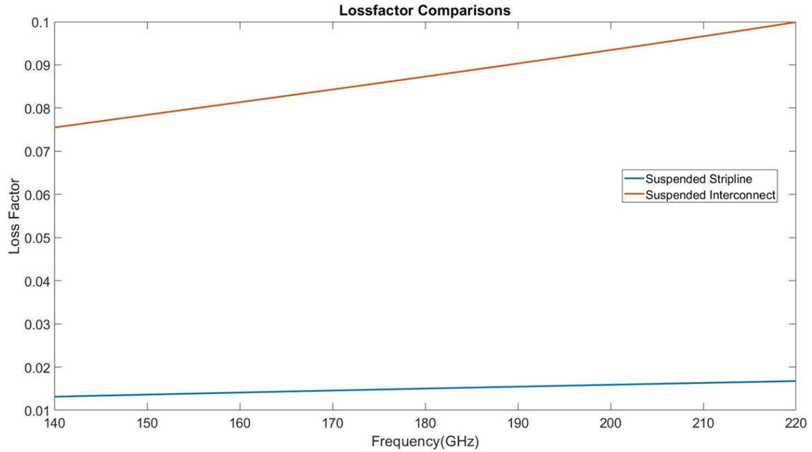
Figure 3.22: Lossfactor simulation comparison of suspended stripline and interconnect.
