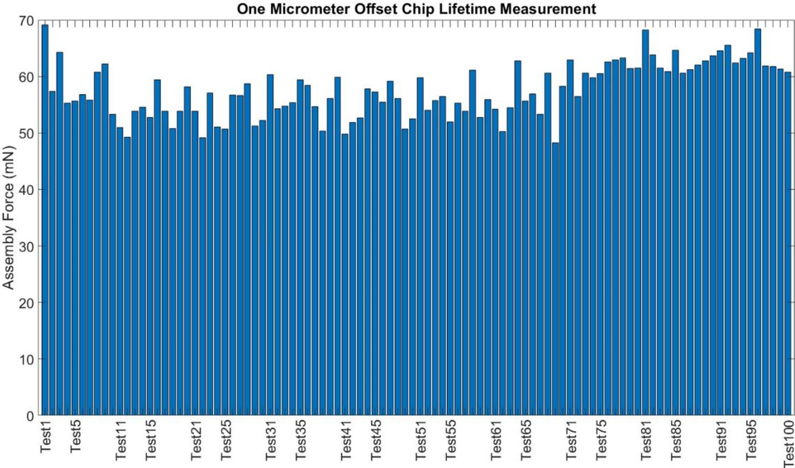
Figure 2.51:Lifetime test of 1  $\mu\text{m}$  offset chip measurement
