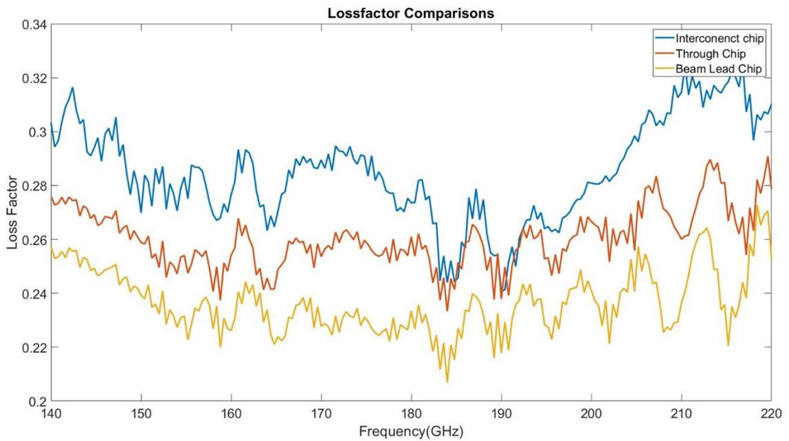
Figure 3.38: Interconnect chip, through chip and beam lead chip loss factor comparison.
