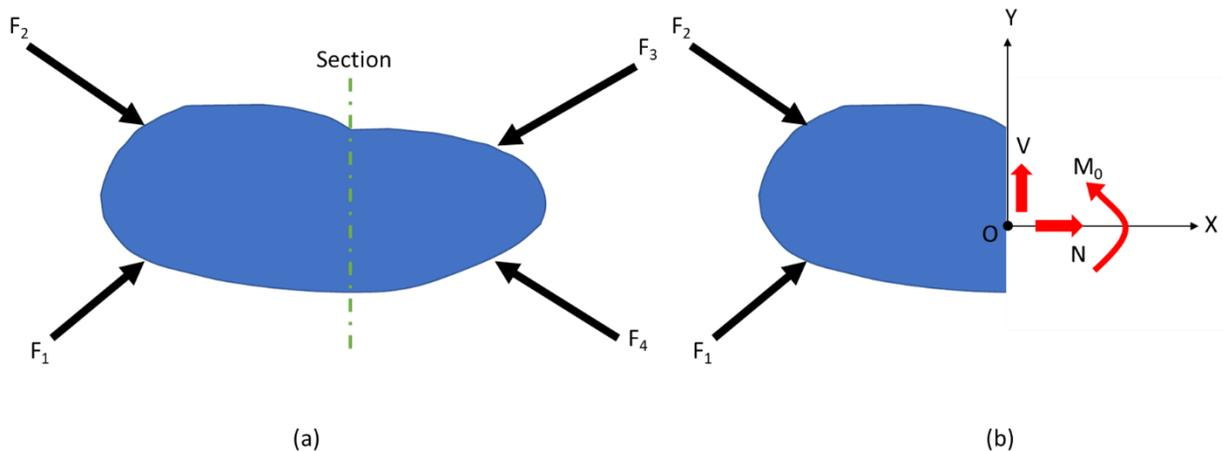
Figure 2.2: Body under external forces (a) and the internal resultant force and bending moment analysis (b).
