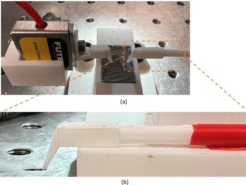
Figure 2.31:(a)Assembly force measurement setup and (b) 3D printed tool for plug chip.
