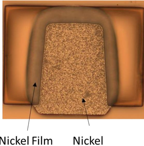
*Figure B. 2: Nickel electroplated on Ti/Au/Ti Seed-layer.*
