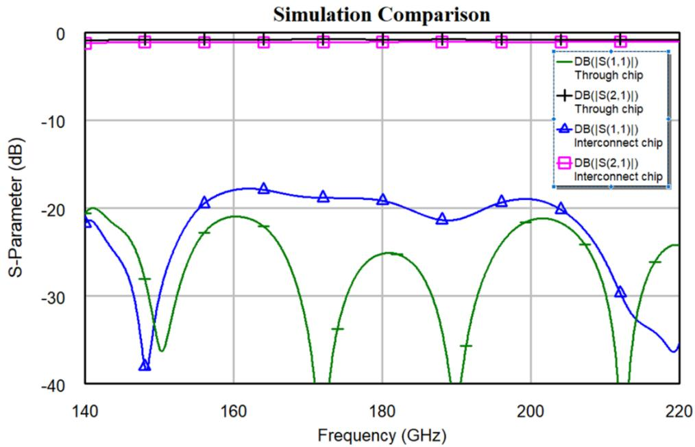
Figure 3.19: Simulation results of through chip and interconnect chip.
