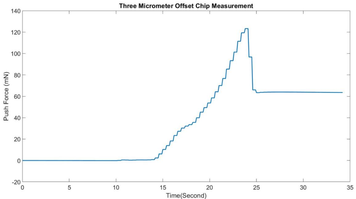
Figure 2.34: 3  $\mu\text{m}$  offset chip assembly force measurement.
