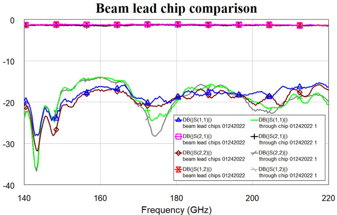
Figure 3.34: Through chip and beam lead chip measurement comparison.
