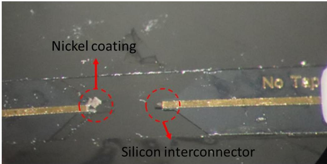
Figure B. 4: Nickel coating peeled off during assembly process.
