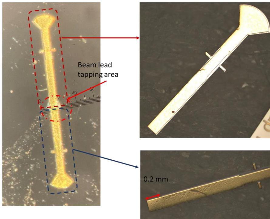
Figure 3.33: Assembled beam lead chips and separated beam lead chips
