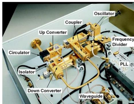
Figure 1.3: Photo of sub-millimeter wave system [25].
