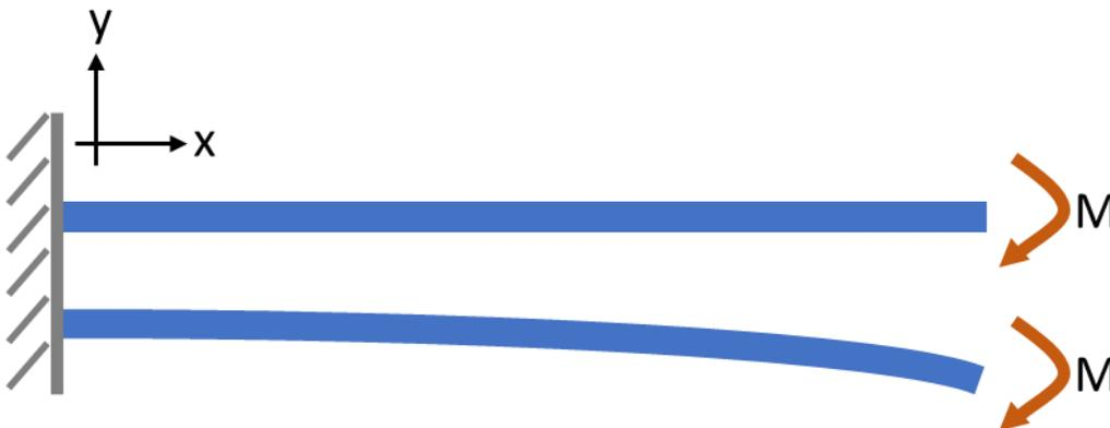
Figure 2.6: Fixed beam before deformation and after deformation.
