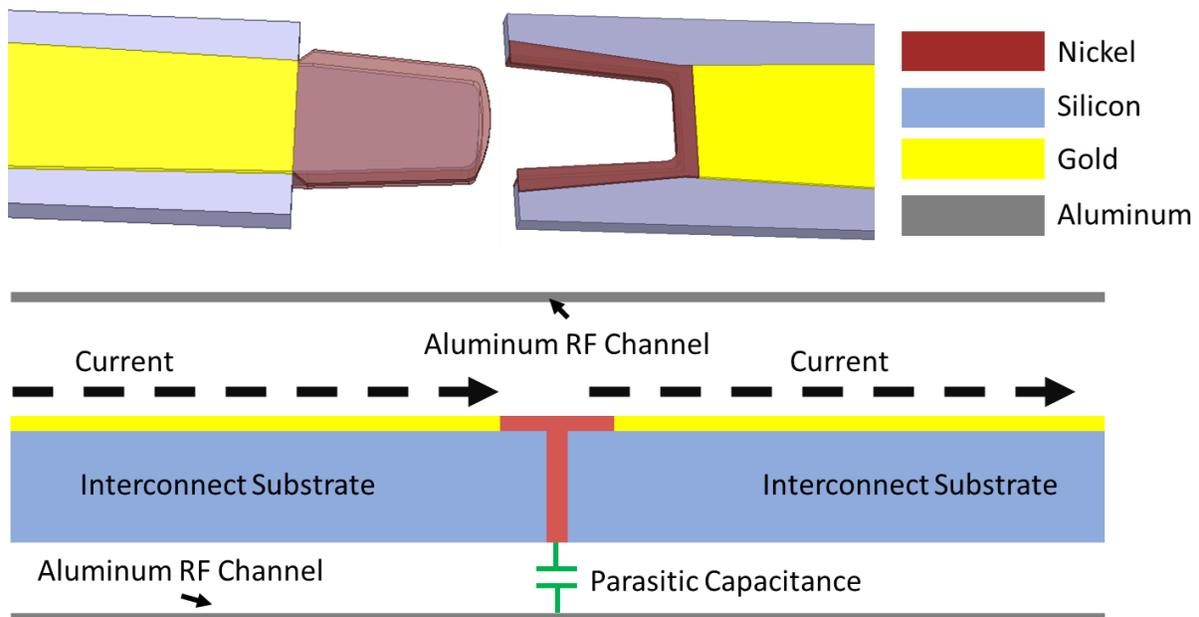
Figure 3.11: Chip to chip interconnect non-flipped assembly and current flow.
