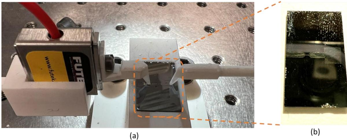
Figure 2.33:(a) Assembly force measurement setup and (b) alignment wafer.
