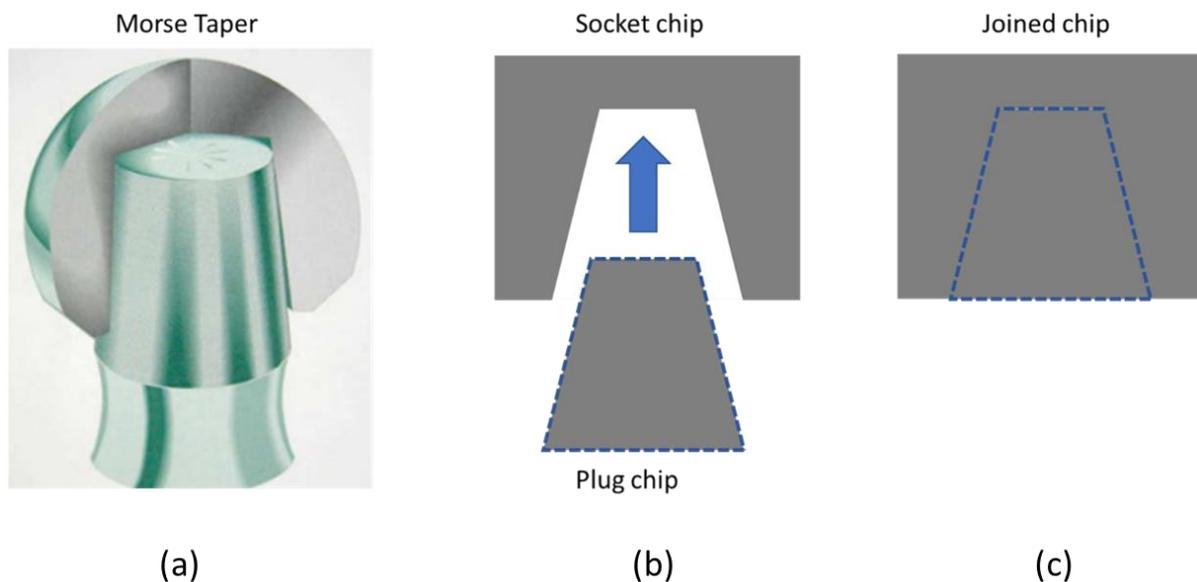
Figure 2.18:(a) Morse taper original application [52](b) Morse taper concept on chip-to-chip interconnect before assembly (c) Morse taper concept on chip-to-chip interconnect after assembly.
