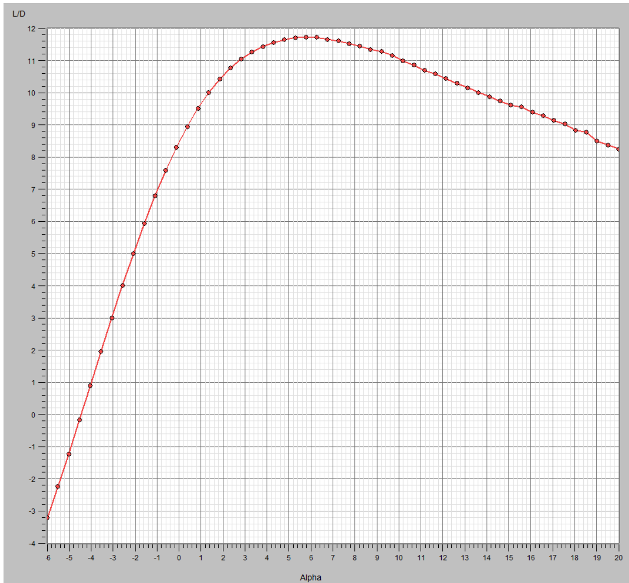
Figure 14: L/D For -6° to 20° AoA
