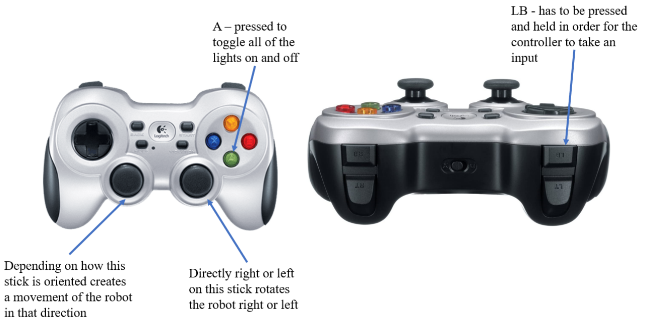
Figure 13. Control scheme for ROSIE
