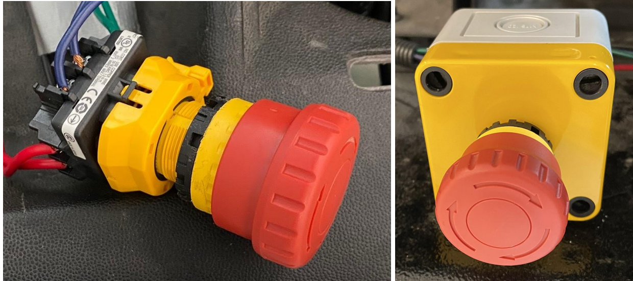
Figure 11. Emergency stop buttons present around the cart to safely shut down the cart when pressed
