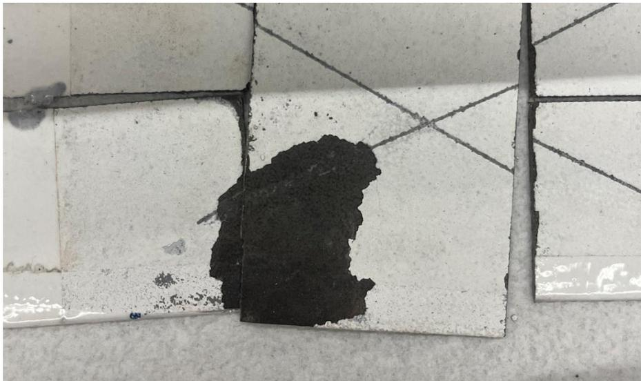
**Figure A8.** Delaminated HTB3 and ZC coating from scribed coupon.
