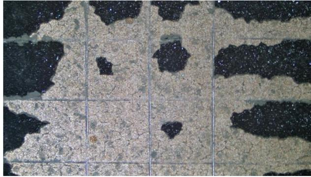
**Figure 11.** ASTM D3359 crosshatch adhesion test of HTB2 coating matrix.
