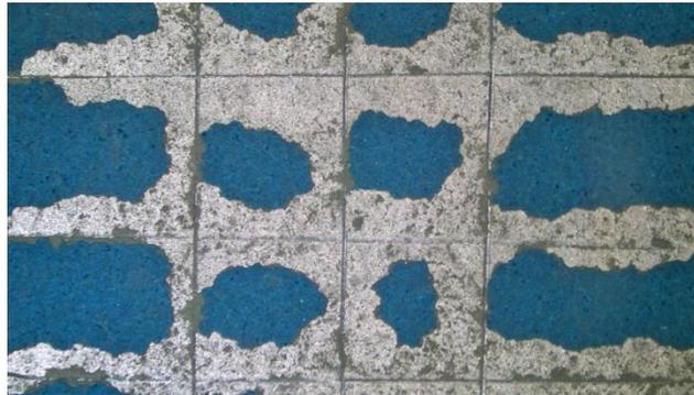
**Figure 10.** ASTM D3359 crosshatch adhesion test of HTB1 coating matrix.
