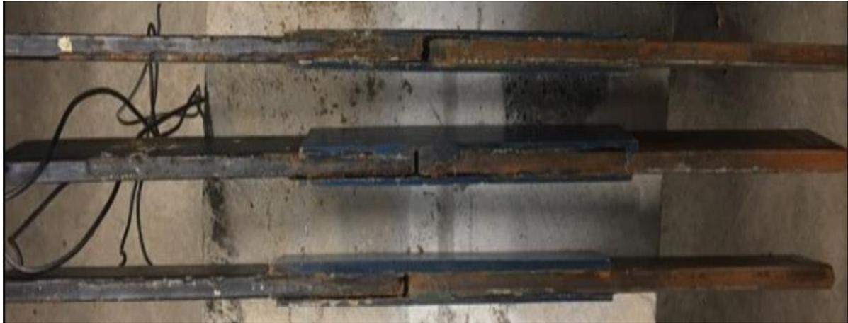
**Figure 27.** Corrosion damage of edges of BL75-B
