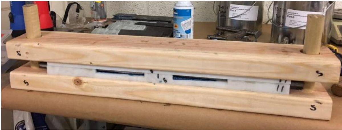
**Figure 17.** Placing the mold into the clamping assembly
