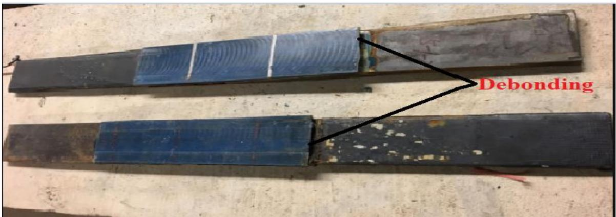
**Figure 44.** Debonding failure
