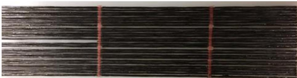
**Figure 1.** Small-diameter CFRP strand sheet
