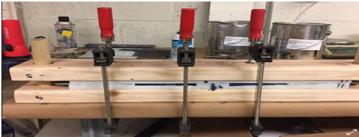
**Figure 18.** Applying pressure to molds by clamping
