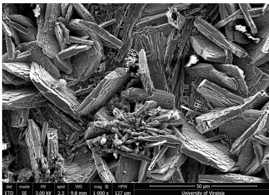
**Figure 5.8:** SEM image Cu(TCNQ) growth on Cu foil in acetonitrile solution of TCNQ at 40 °C for 4 h.
