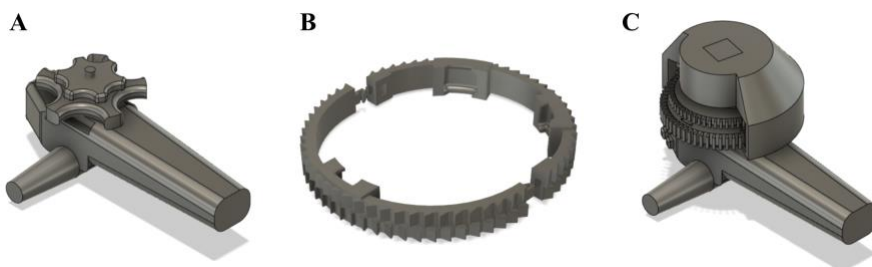
Fig. 1. Initial CAD prototype of solution. (A) A CAD rendering of the classic Olympus CF-140S colonoscope model limited to the proximal handle portion. (B) The original dial mask used in the first iteration of the prototype that features two snap-together clamps to secure the mask onto the dial of interest. (C) A CAD rendering of the first medical device solution featuring a ratcheting mechanism housed in a casing on top of the endoscope dials.
