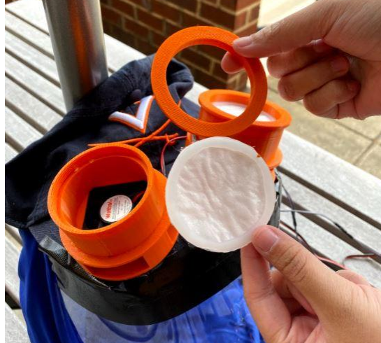
Figure 12: Removable Filter Material and Top Section of Fan Casing
