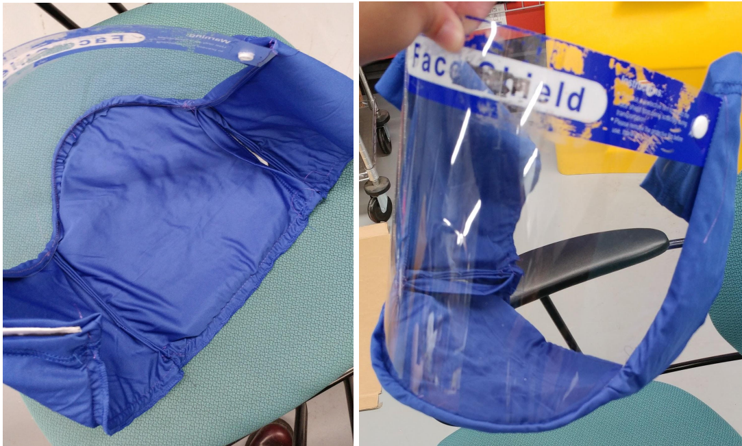
Figure 15: Final curved neck piece design with pockets
