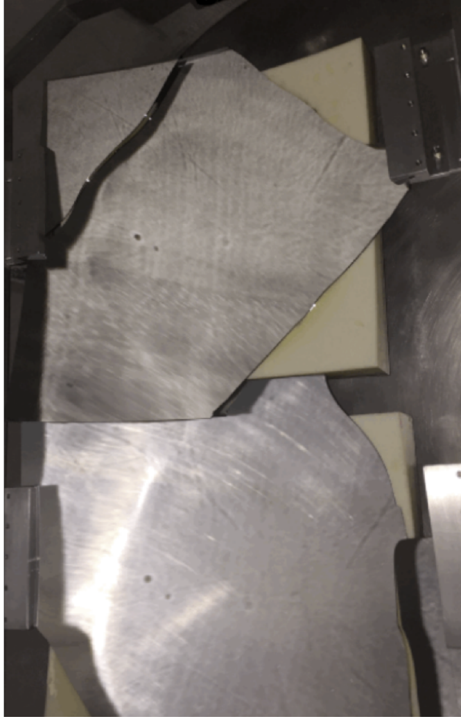
Figure 4-15: A picture of the broken HMS Cherenkov mirrors taken after the detector was removed from the hut for repair. The mirrors' Rohacell supports are visible where portions of the mirrors have broken off.
