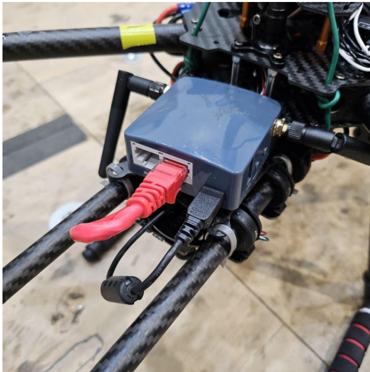
Figure 21. Onboard modem for Raspberry Pi
