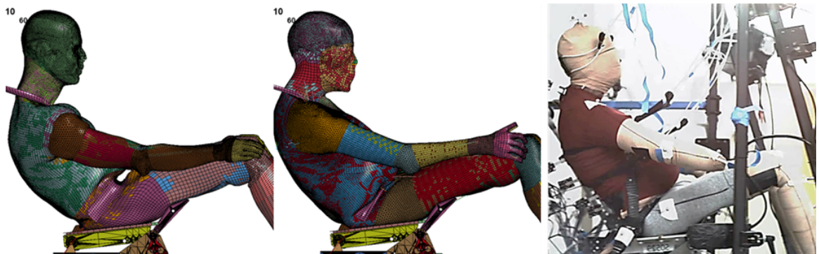
Figure 4.22: Lap belt-flesh interaction during forward pelvis displacement. Left-right: GHMBC, THUMS, PMHS.
