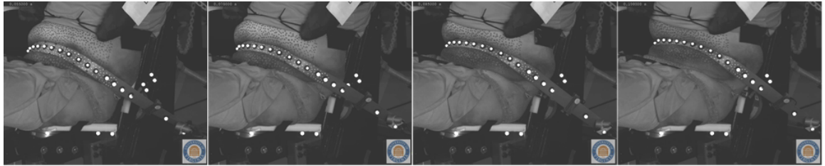
Figure 5.12: Lap belt interaction with abdominal soft tissue for subject 993M's test (D1592) at 55 ms, 70 ms (time of initial peak in lap belt tension), 85 ms (second peak), and 100 ms.
