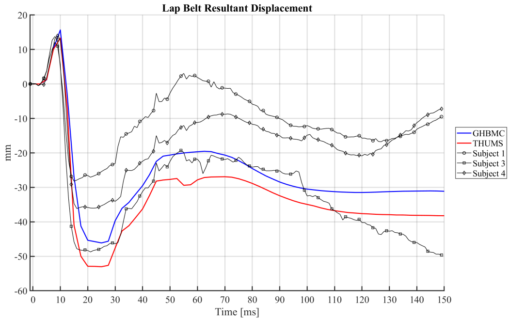
Figure C.21: Lap Belt Resultant Displacement: HBMs (Nominal Pelvis Angle) vs. PMHS
