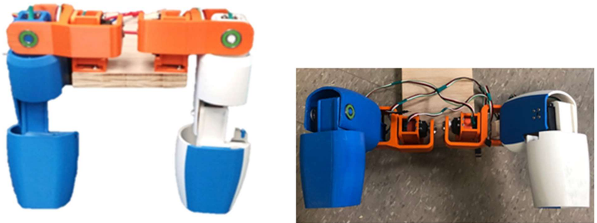
Figure 26: Final prototype of arm subassembly. Left image shows the front of the arm subassembly. The right image is a top view of the subassembly.
