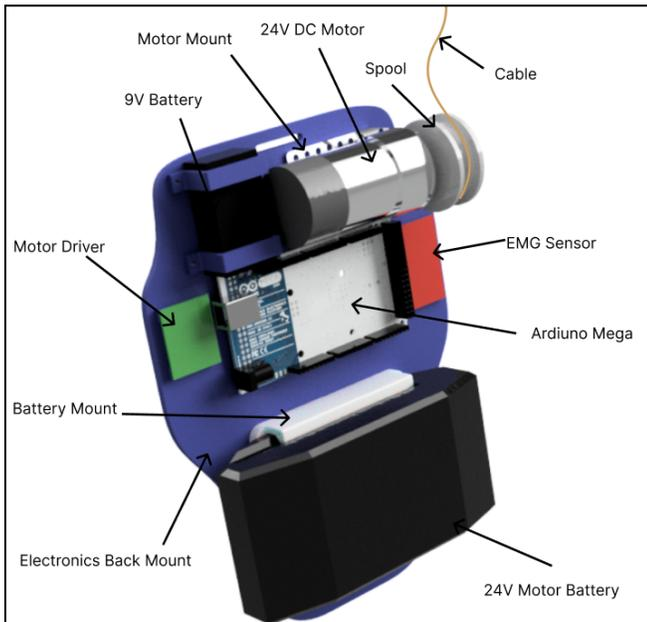
Fig 28. Electronic assembly on back mount
