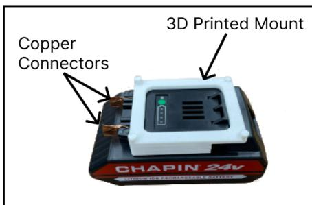
Fig 19. 24 Volt lithium battery shown with 3D printed mount and two copper connectors
