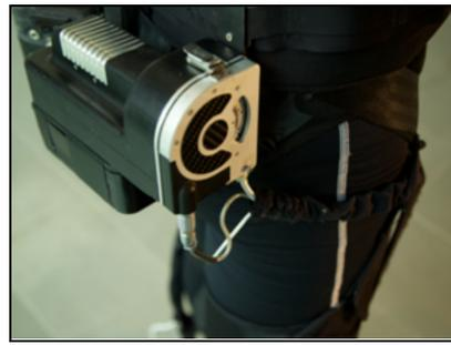
Fig 3. Bowden Cable Mechanism [10]
