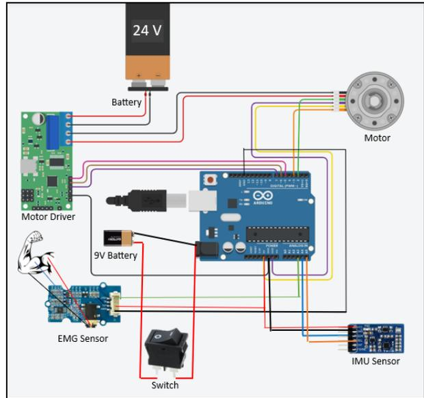
Fig 29. Circuit diagram of the final design
