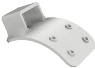
Fig 25. Improved wrist mount CAD design
