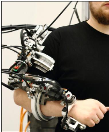
Fig 1. Seven degree of freedom (DOF) exoskeleton [9]
